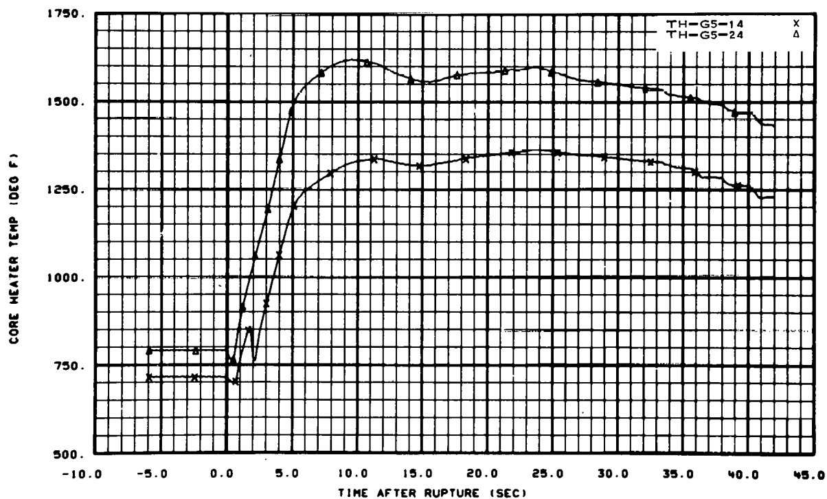
Fig. 64 Core heater temperature, Rod G-5.
