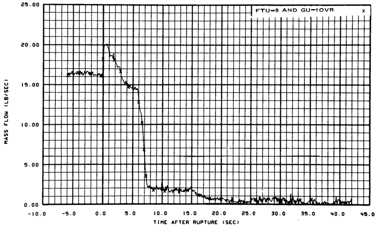
Fig. 135 Mass flow in intact loop (FTU-9 and GU-10VR).
