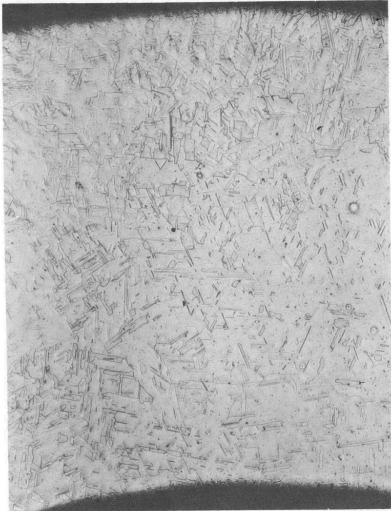
Fig. 16. Type 347 Stainless Steel Boiler Two Coils from Bottom (cold end about 350° F)
