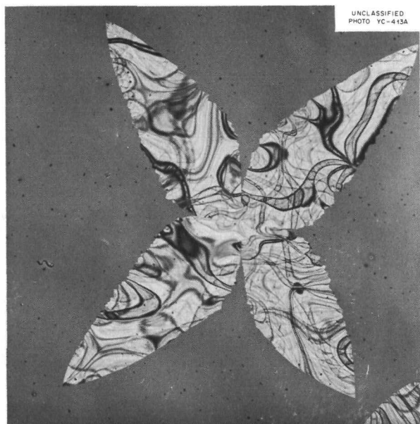
Fig. 2.3. Electron Micrograph of a Thermally Recrystallized Region in a 225-A Anodic Film Stripped from a Tantalum Specimen and Annealed for 18 hr at 600°C. 7400X. Reduced 58.5%.
