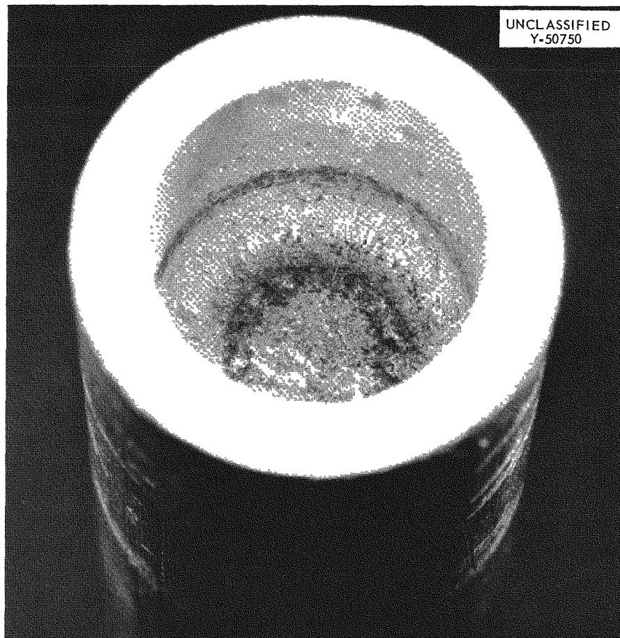
Fig. 30.4. Brazed End Closure in Aluminum Tube. Good filleting and flow of the brazing alloy are evident.
