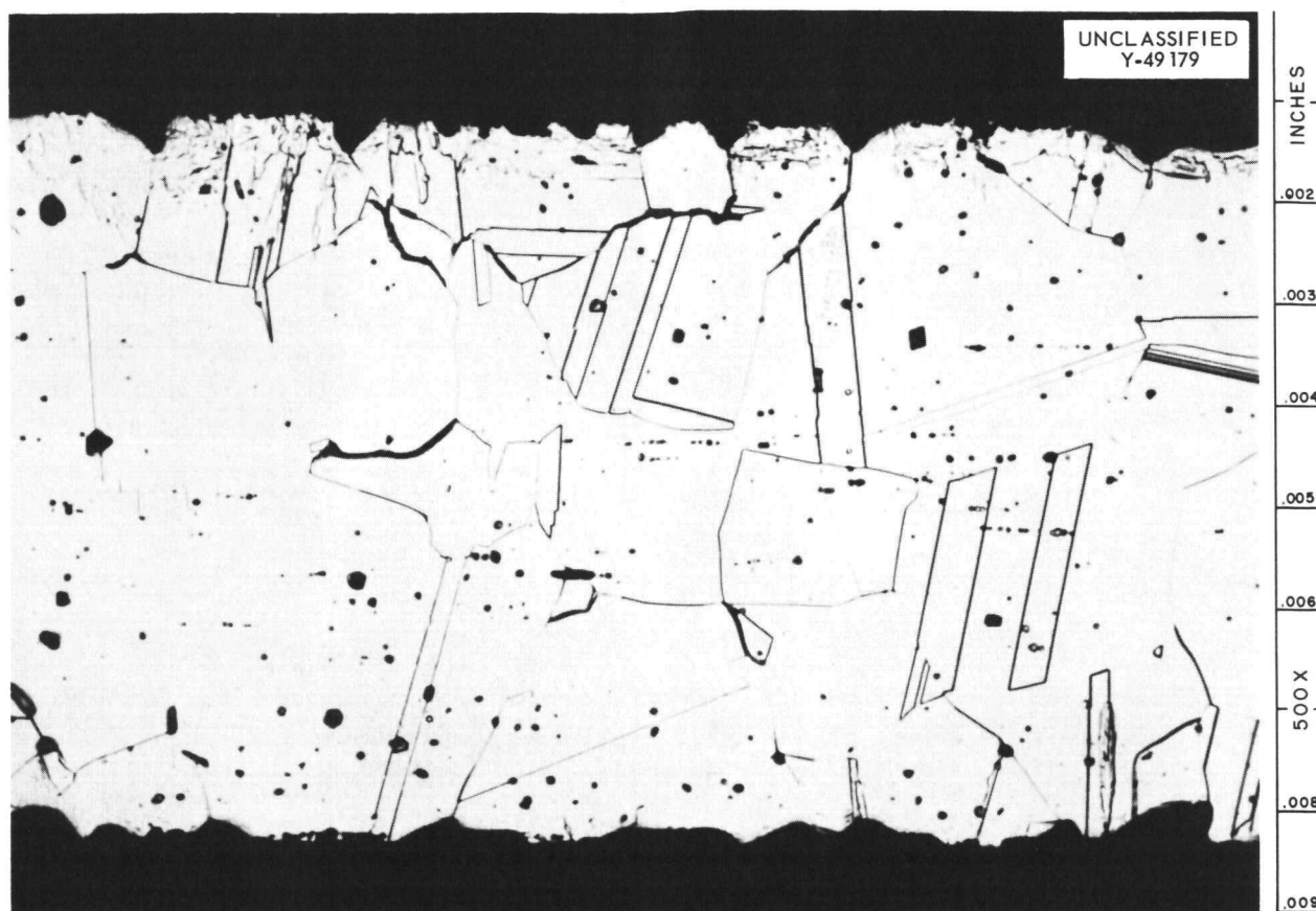
Fig. 19.8. Type 316 Stainless Steel Oxidized in Air at 820°C (1500°F) and Subsequently Evaporated at 1800°F (982°C) at 5 \times 10^{-7} torr. Etchant: glyceria regia.
