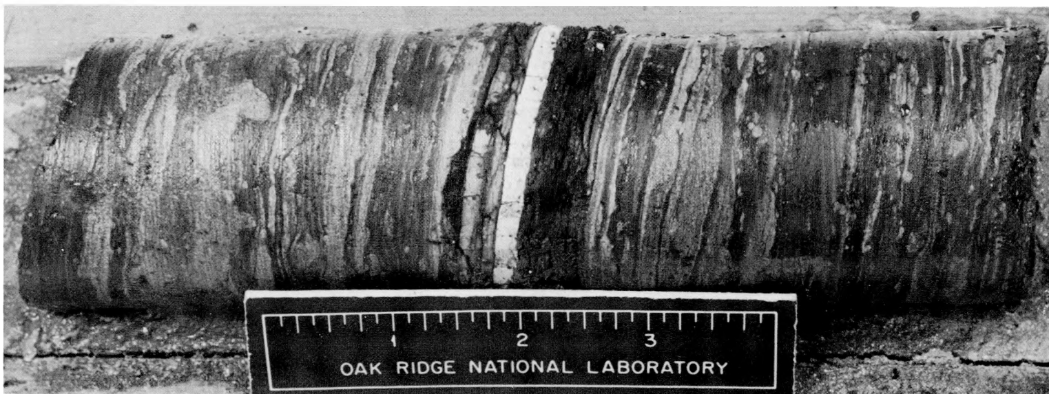
Fig. 1.59. Core Containing Grout Seam from Well 345 ft NW of Injection Well.
