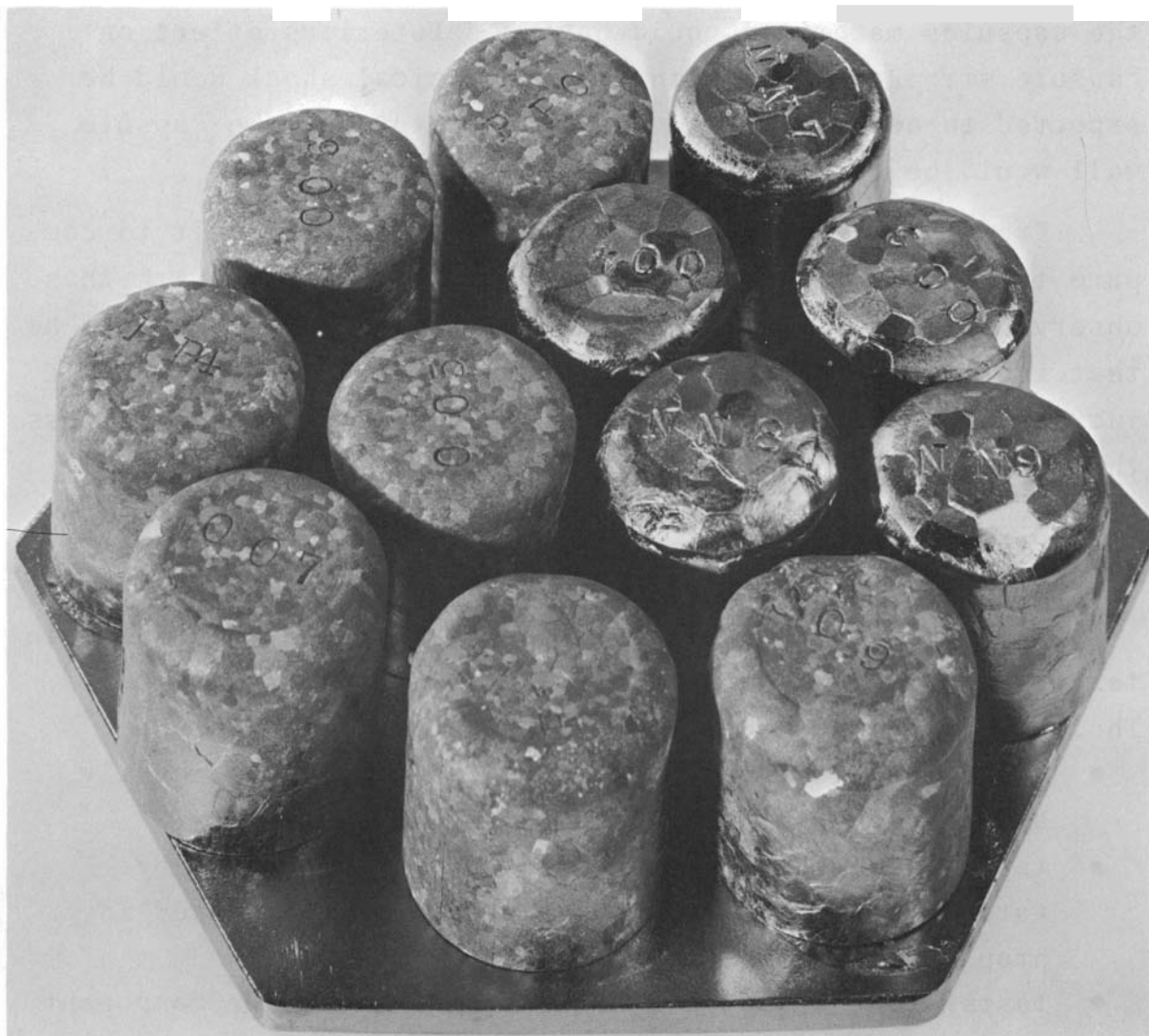
FIGURE 20. Tantalum and Ta-10%W Couples of \text{Sm}_2\text{O}_3 Tested at 2000 °C for 3000 hr - Before Sectioning
