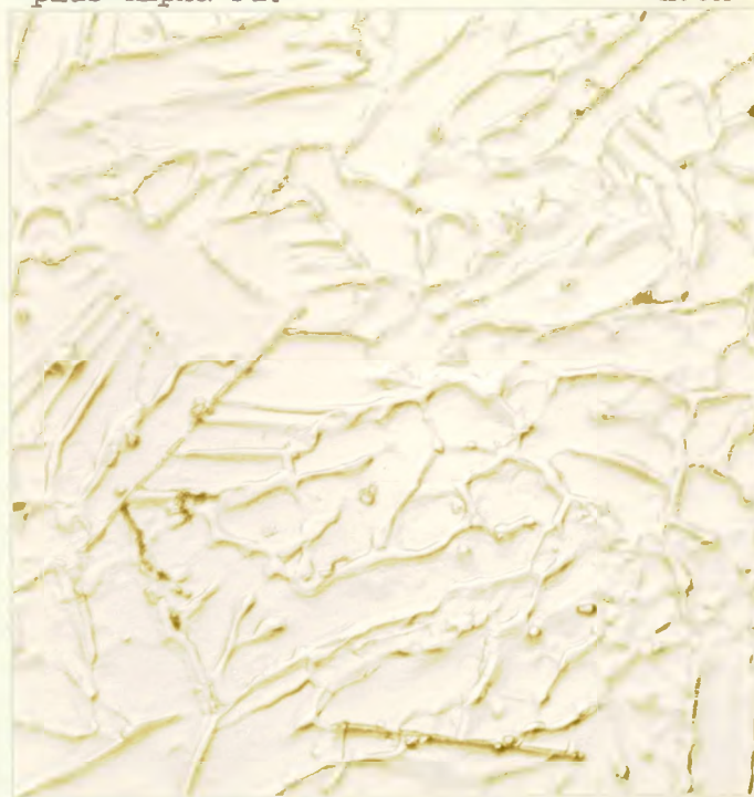
Fig. 8. Cast Pu + 8 a/o Al. Etched by cathodic bombardment. Cast structure of delta plutonium. 500X
