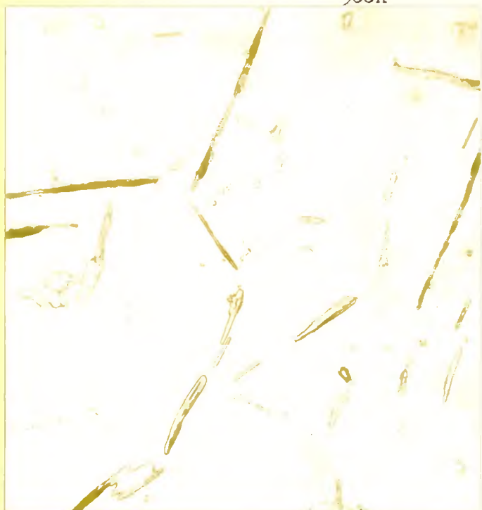
Fig. 15 Plutonium + 5 a/o C. Same specimen as Fig. 14, but a different area. Same electropolish. Some PuC present, but acicular compound presumed to be a complex compound in an alpha Pu matrix. 500X
