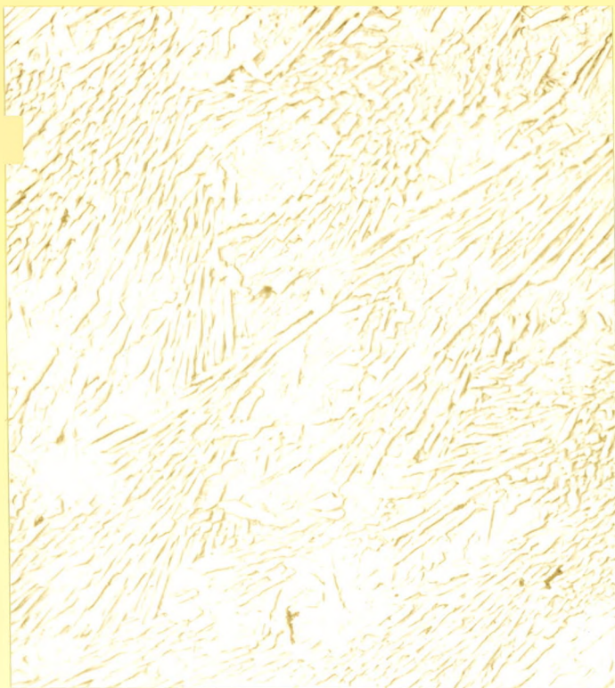
Fig. 17 Plutonium + 10 a/o Ru. Electro-etched 10 sec at 8 V in Sol. 1. The eutectic microstructure consists of Pu 3 Ru in alpha plutonium. 500X
