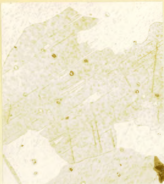
Fig. 5 Same specimen as Fig. 4. Electro-etched 20 min at 14 V plus 2 min at 6 V in Sol. 3 and photographed using polarized light. Fine detail and sharp delineation of grains is shown. 250X
