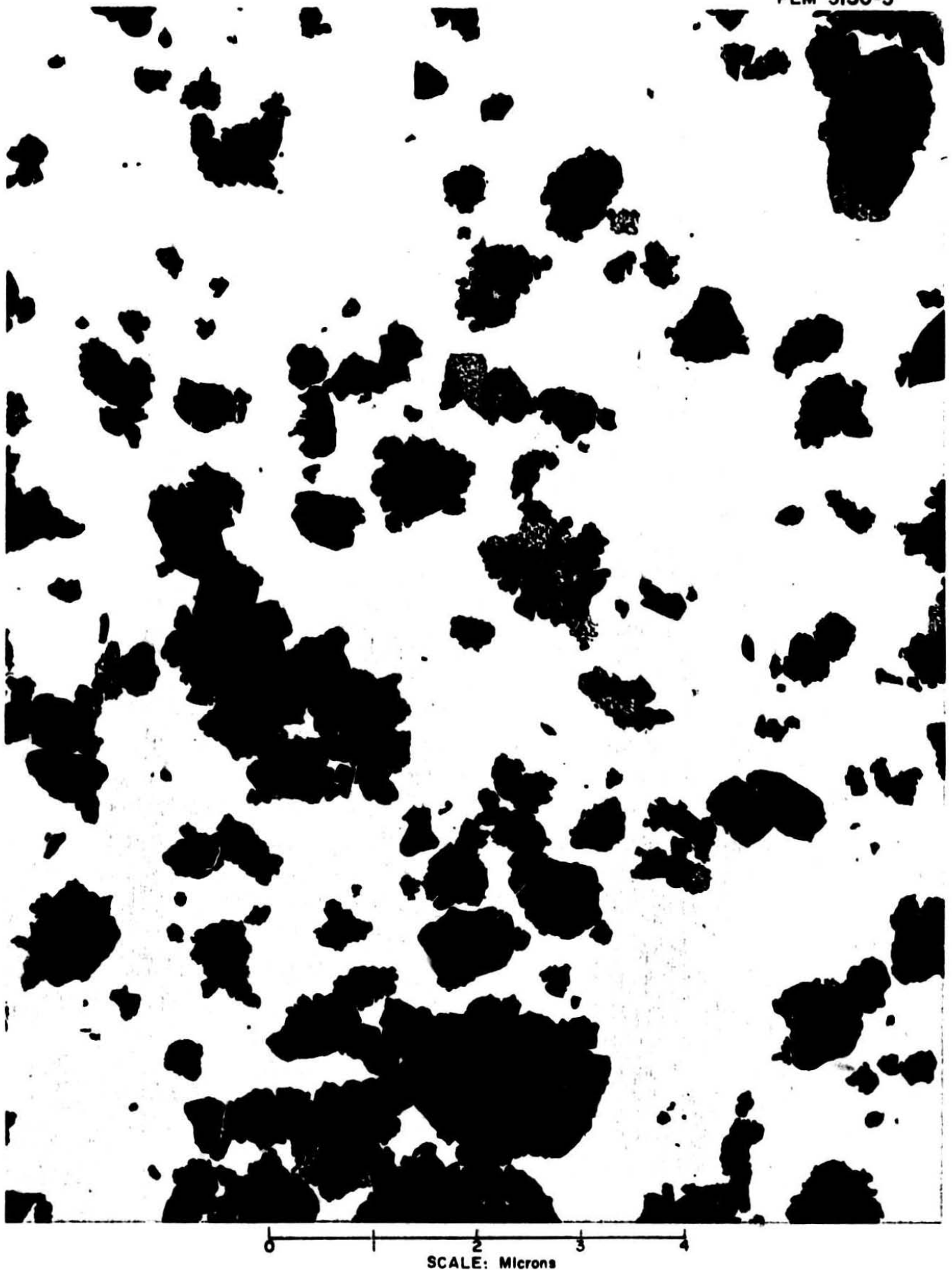
Fig. 3. Solids from cyclone pot, run TU-1. 20,000 x
