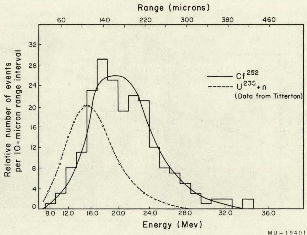
Fig. 2. Energy spectrum of long-range alpha particles associated with fission.  $\text{Cf}^{252}$ ,  $\text{U}^{235} + n$  (Data from Titterton et al. <sup>24</sup>).
