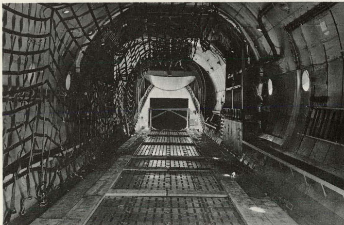
Figure B-55 Separators used between shoring; power conversion mockup ready for loading
