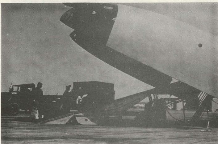
Figure B-92 C-124 loading ramp (note clam-shell doors) during preparations for loading power conversion mockup
