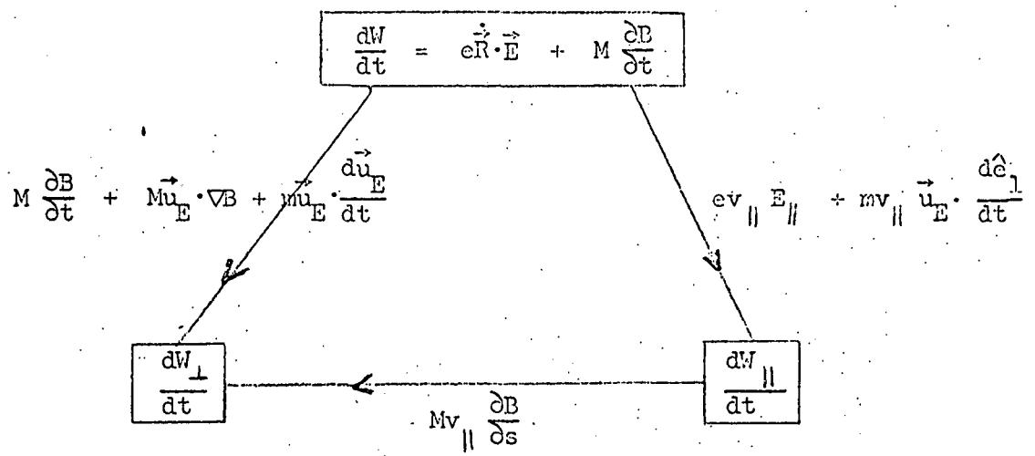
Fig. 3. Energy changes in a time-dependent field.
