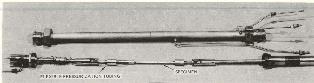
Figure 2. Test Assembly for 1:1 Biaxial Stress-Rupture Tests
