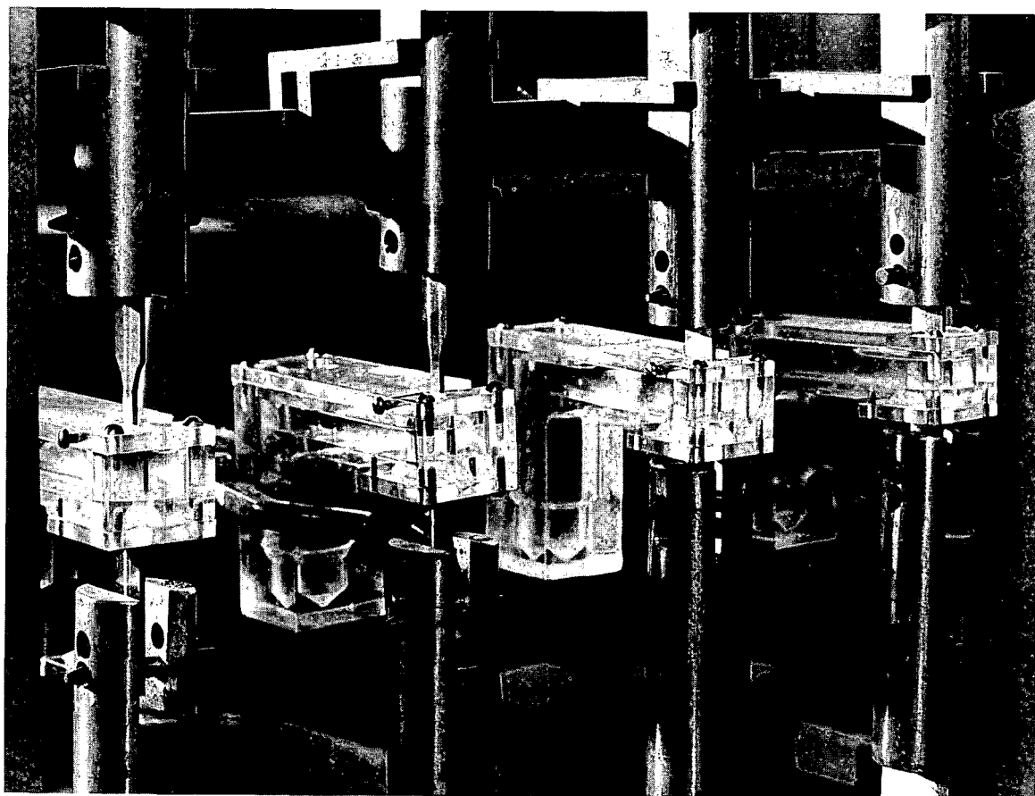
Figure 3. PLEXIGLAS ENVIRONMENTAL CELL FOR TENSILE-TYPE STRESS-CORROSION SPECIMENS.
