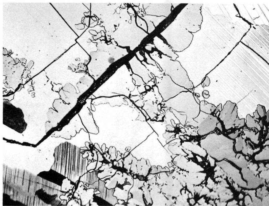
FIGURE 21. URANIUM-8.8 w/o CARBON ALLOY AFTER HEATING 1000 HR AT 1100 C
