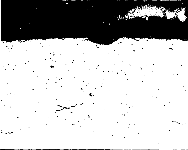
Figure 9 - Longitudinally-oriented groove found on the OD surface of fuel rod 837. As-polished 200X
