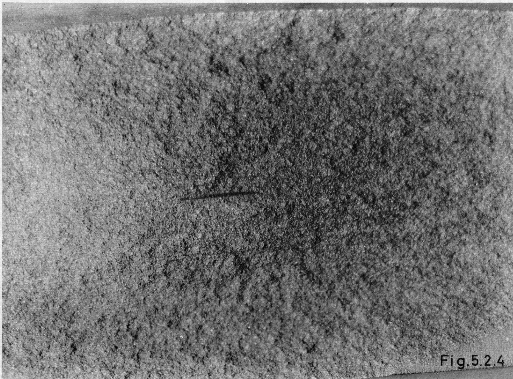
FIG. 5.2.4 SPALLED ROD WITH FAULT
