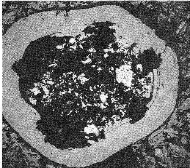
Fig. 27 HPD5/5A; Penetration of Spearhead Attack into Outer Columnar Coating (X154)
