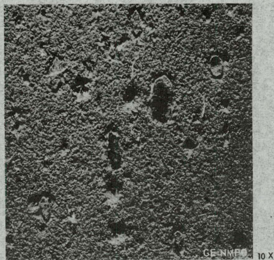
(b) Agglomerated W in presintered W-25Re powder compact
