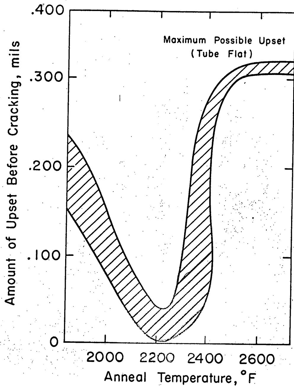
Fig. 8 - Upset before cracking of tungsten rings (0.440 inch OD, 0.035 inch wall) vs. temperatures of annealing for one hour. Tungsten tubes extruded at 2200°F. Test temperature 700°-1000°F.
