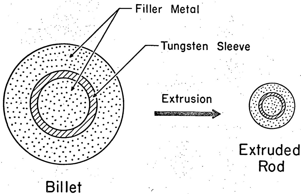
Fig. 2 - Filled Billet Method of Extrusion
