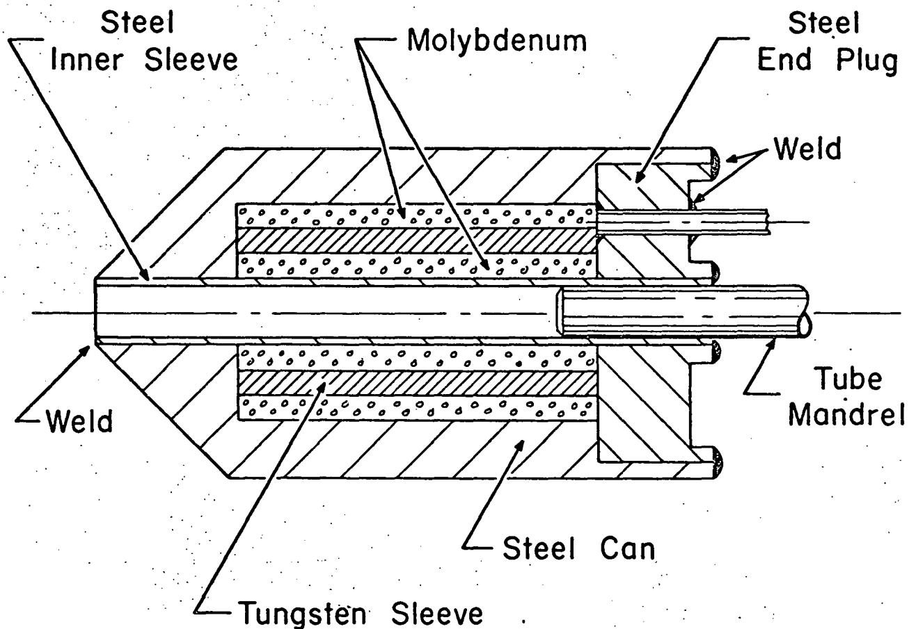
Fig. 6 - Billet for 2200°F Extrusion of Large Tungsten Tubes
