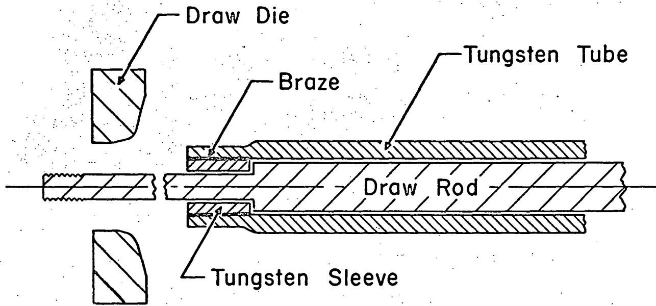
Fig. 7 - Technique Used for Drawing of Tungsten Tubing
