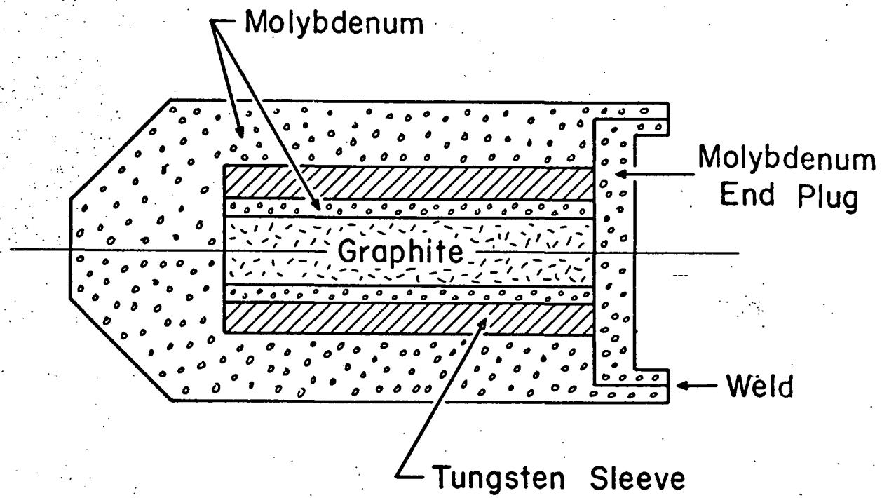
Fig. 4 - Billet for 3300°F Extrusion of Tungsten Tubes
