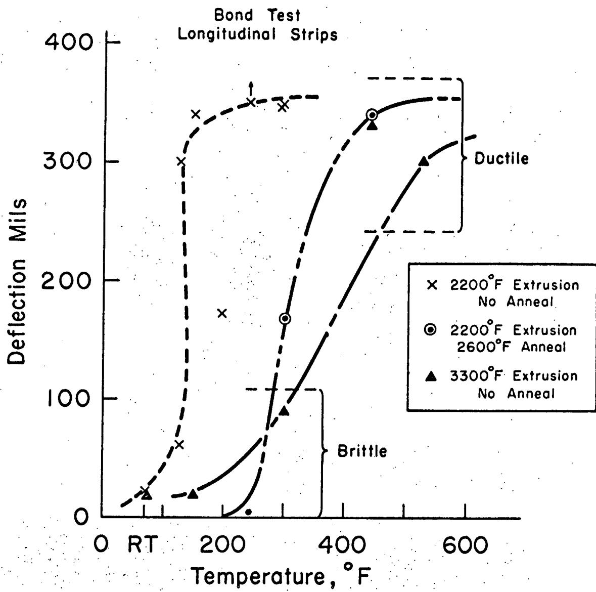
Fig. 9 - Bend test results, tungsten tubing, longitudinal strips
