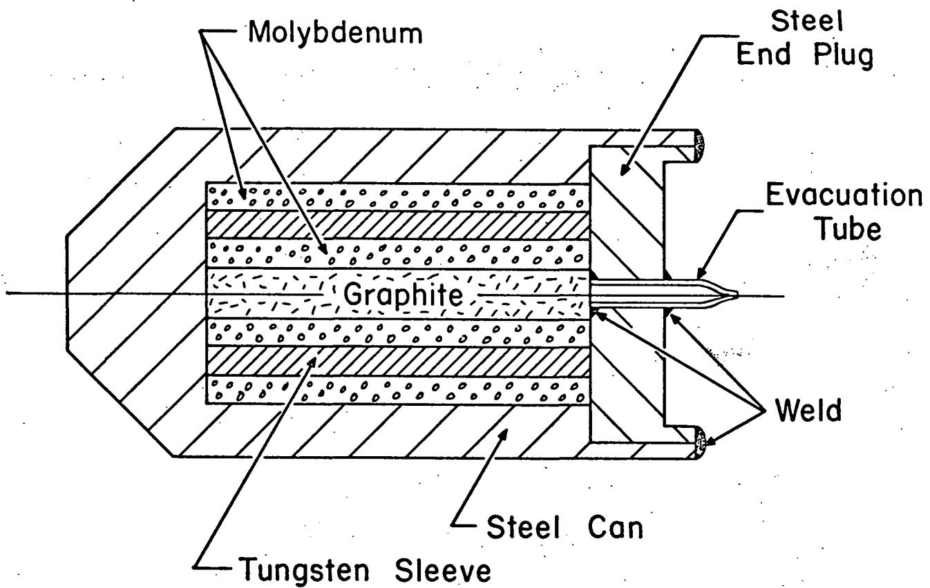
Fig. 5 - Billet for 2200°F Extrusion of Tungsten Tubes
