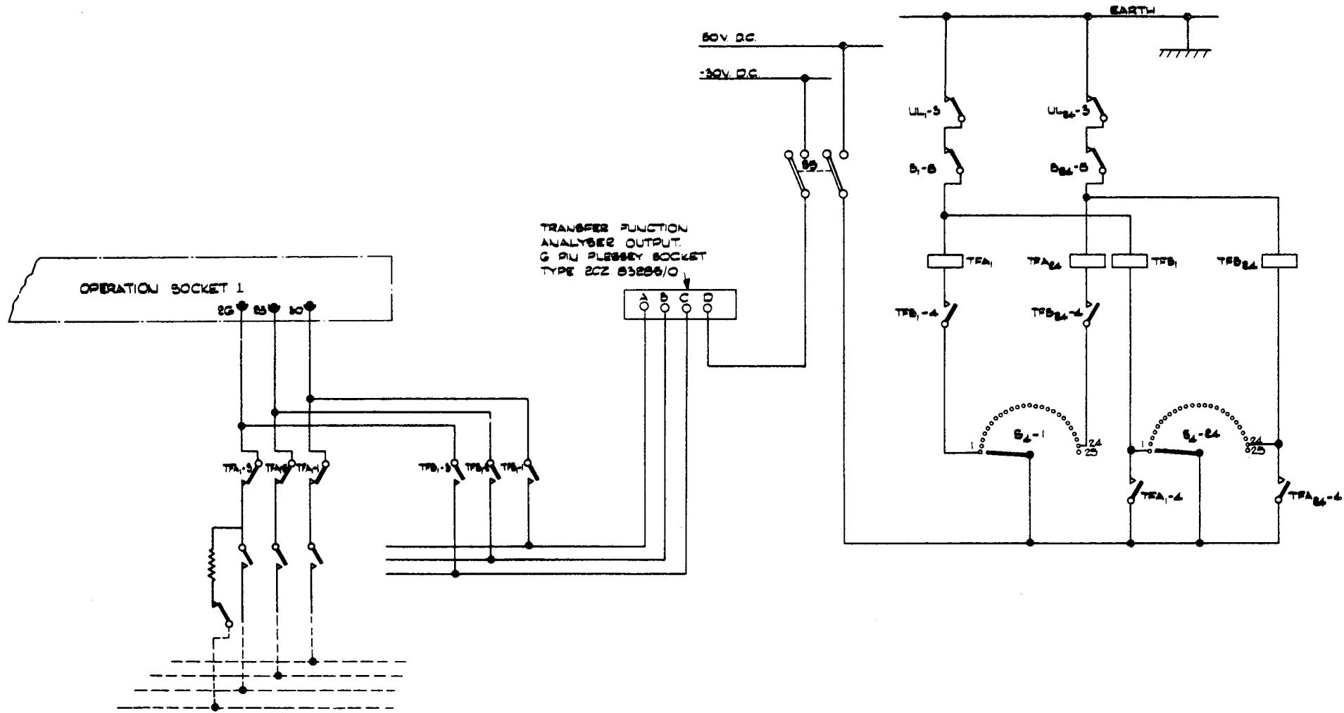
FIG. 22 CIRCUIT FOR TRANSFER FUNCTION ANALYSIS - DRG. NO. CE175
