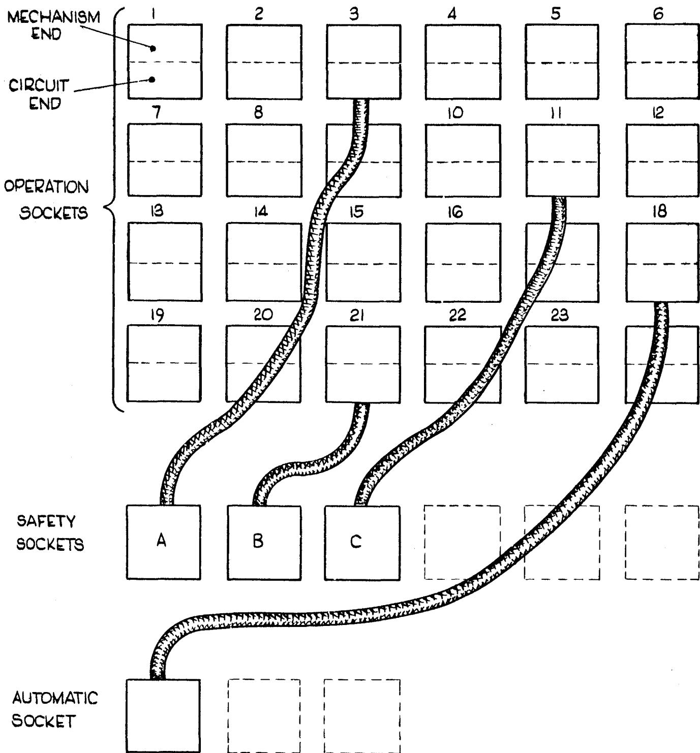
FIG. 8 CONNECTING BOX - SCHEMATIC.
