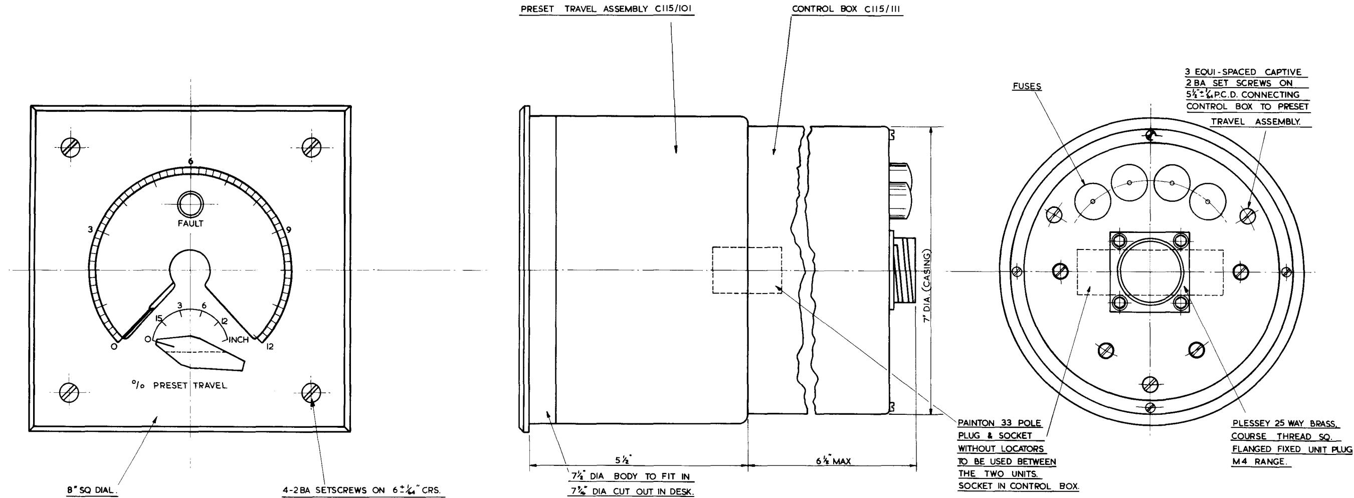
Fig. 13 LIMITED PULSE GENERATOR (OUTLINE) - DRG. NO. C115/110.
