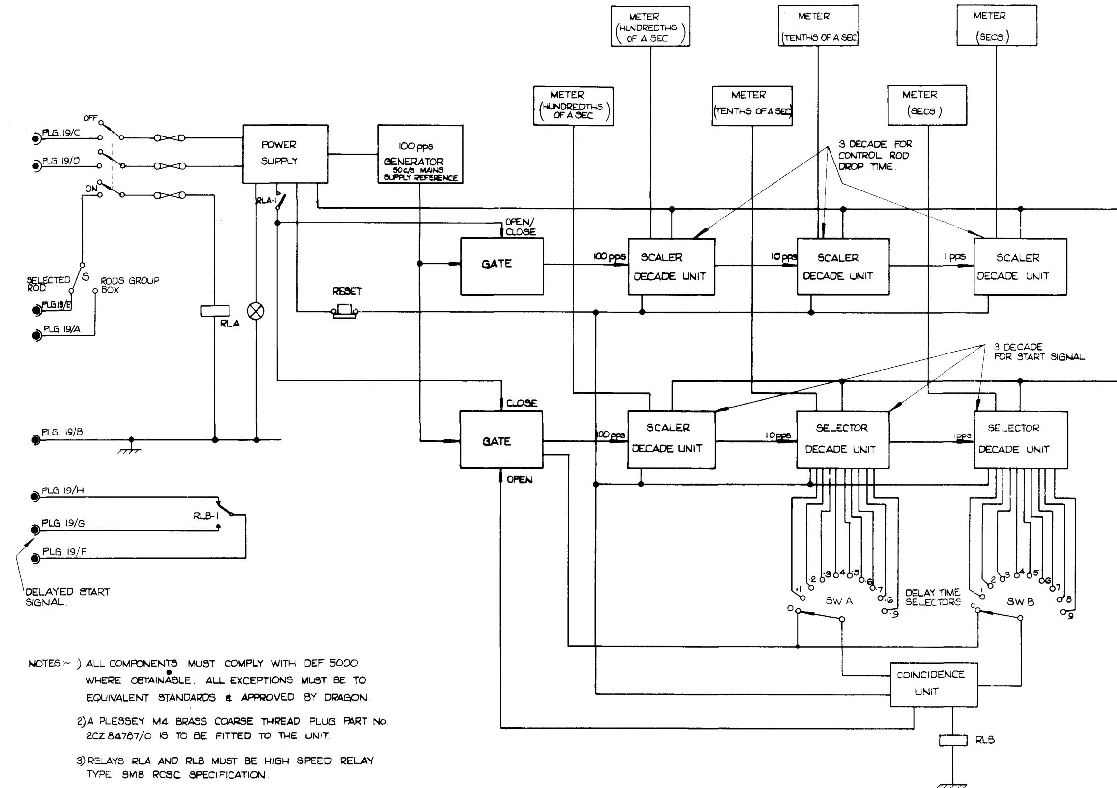
Fig. 20 CONTROL ROD DROP TIMING UNIT - SCHEMATIC - DRG. NO. C116/001
