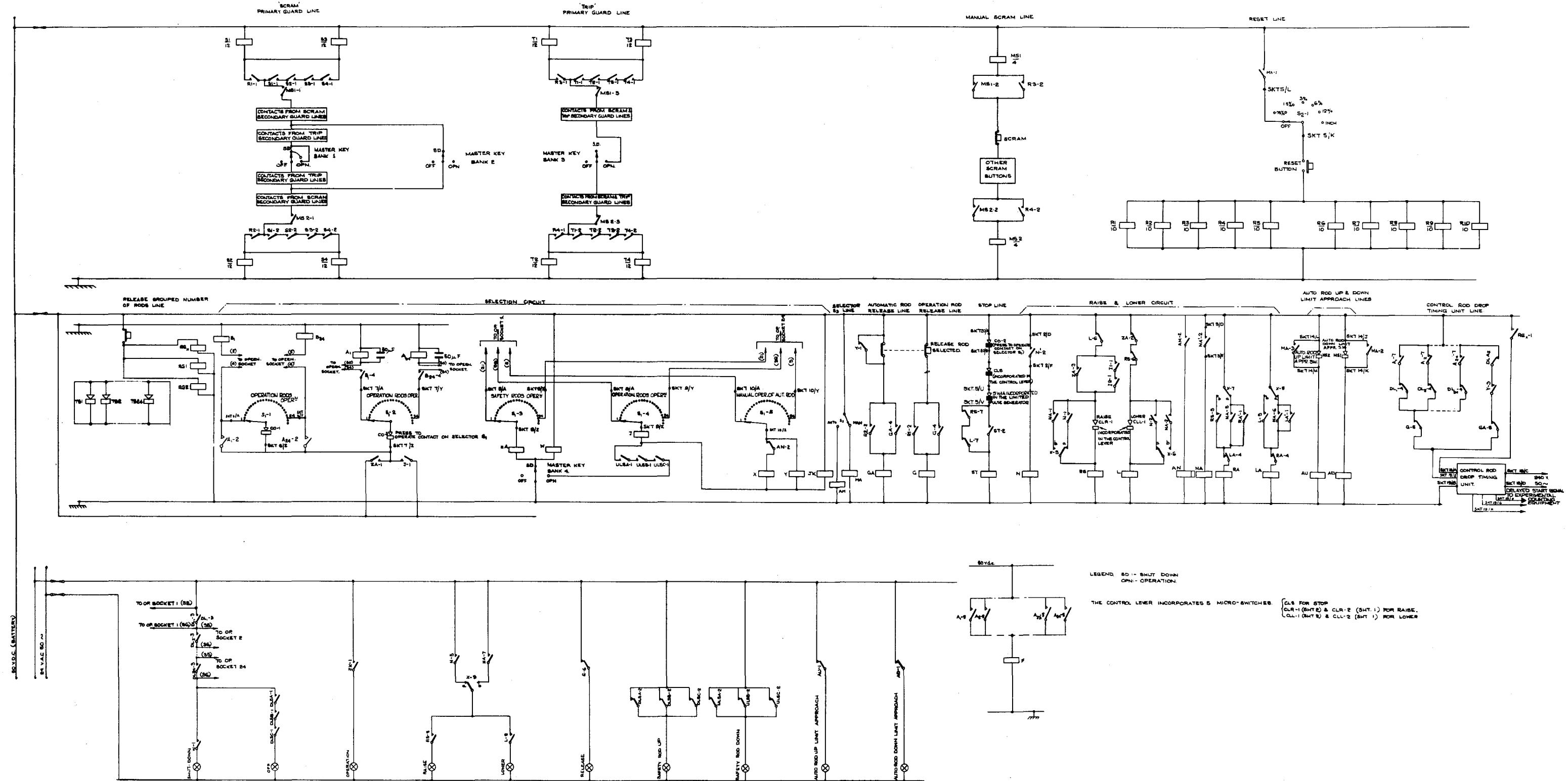
Fig. 3 SCHEMATIC DIAGRAM FOR ABSORBER RODS CONTROL CIRCUIT - DRG. NO. C112/001 SHT. 2.
