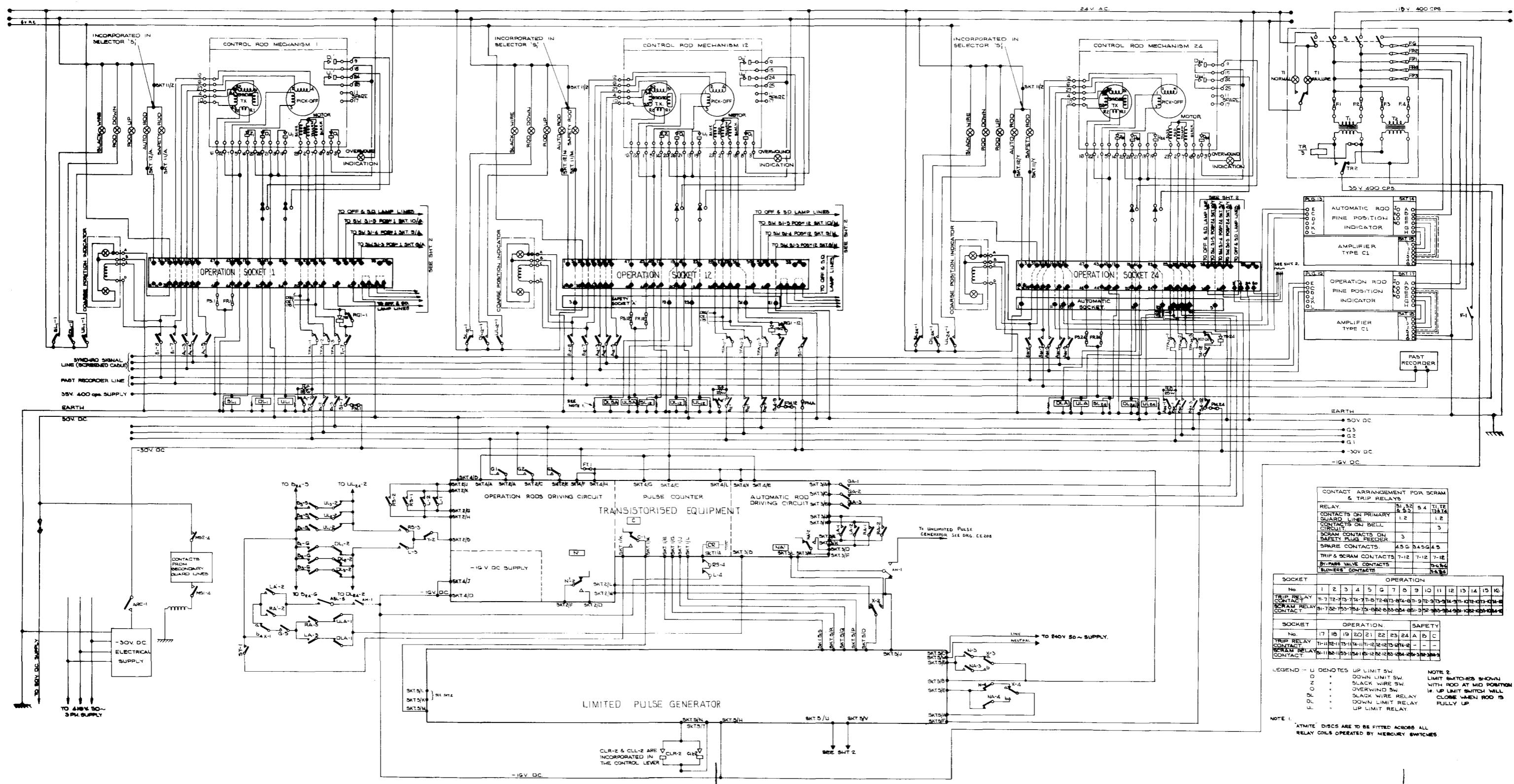
Fig. 2 SCHEMATIC DIAGRAM FOR ABSORBER RODS CONTROL CIRCUIT - DRG. NO. C112/001 SHT. 1.
