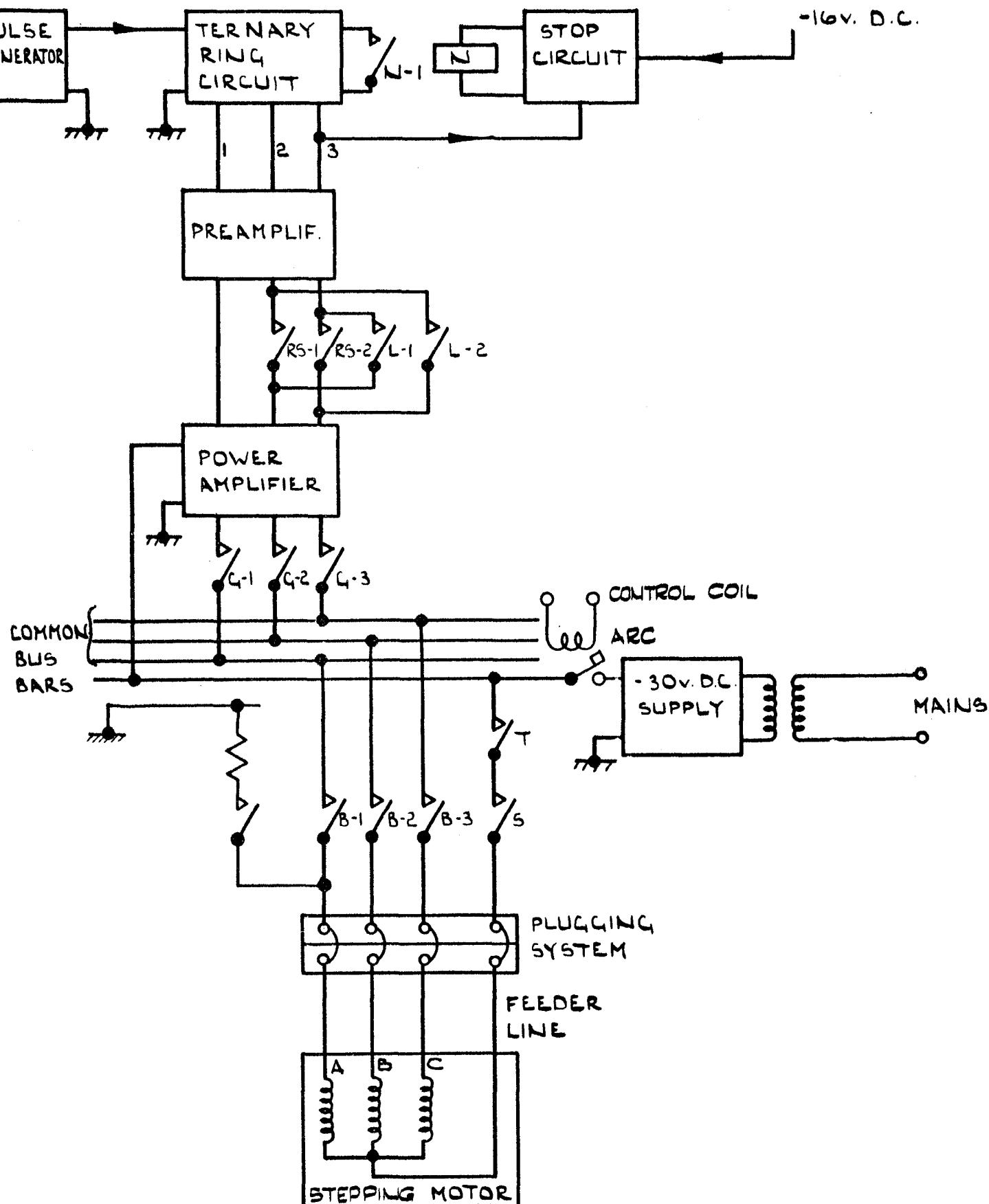
FIG.4 DRIVING CIRCUIT - SCHEMATIC
