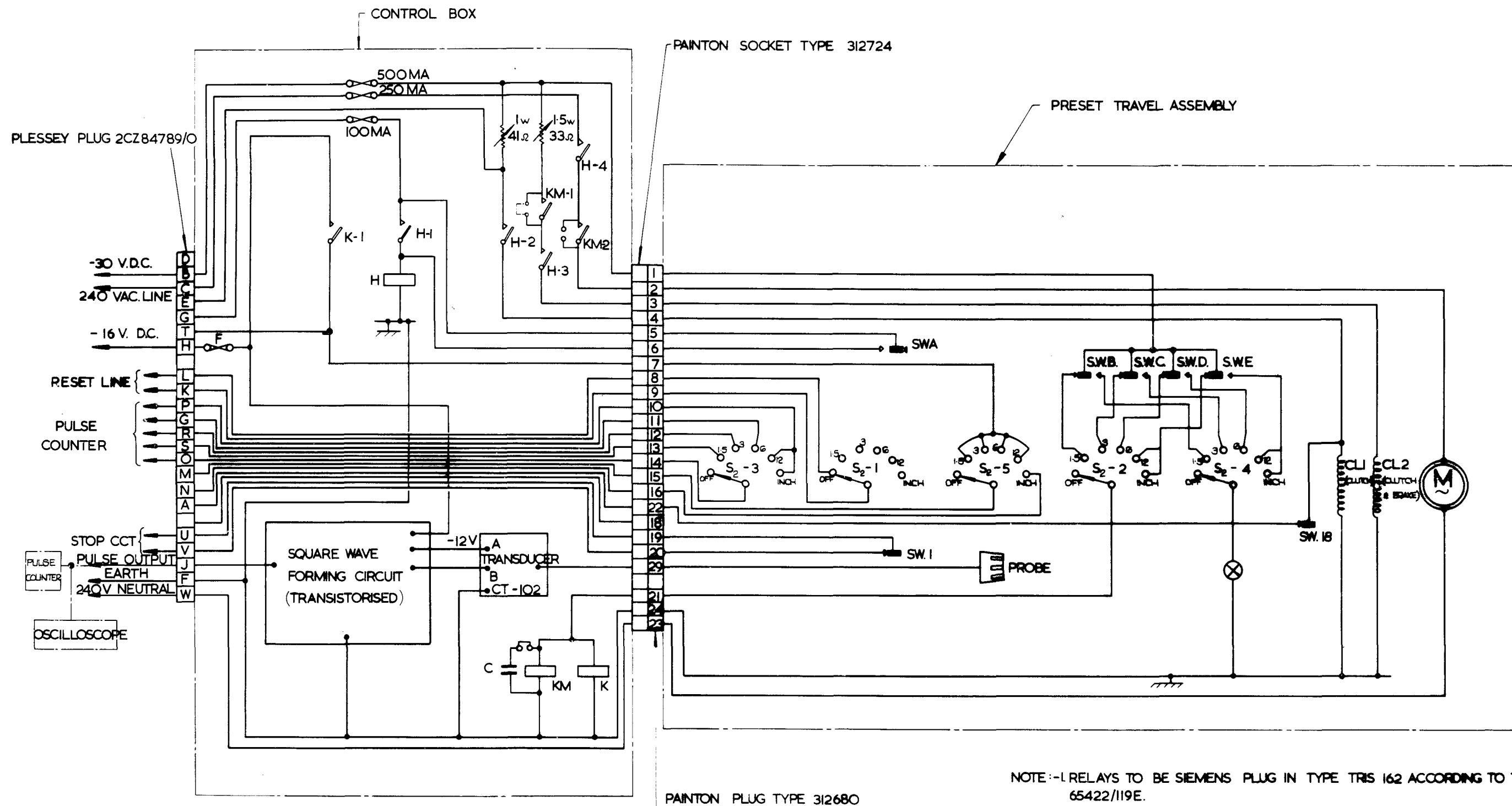
NOTE : -1 RELAYS TO BE SIEMENS PLUG IN TYPE TRIS 162 ACCORDING TO T B V 65422/119E.
