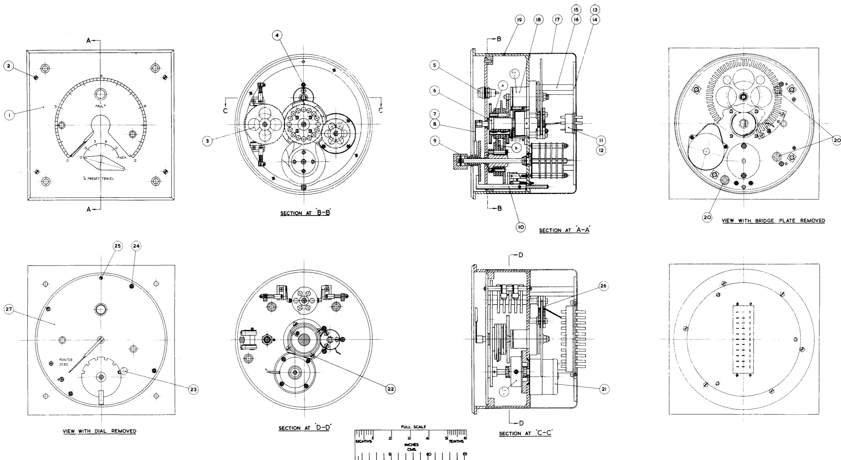
Fig. 14 LIMITED PULSE GENERATOR PRESET TRAVEL ASSEMBLY - DRG. NO. C115/101.
