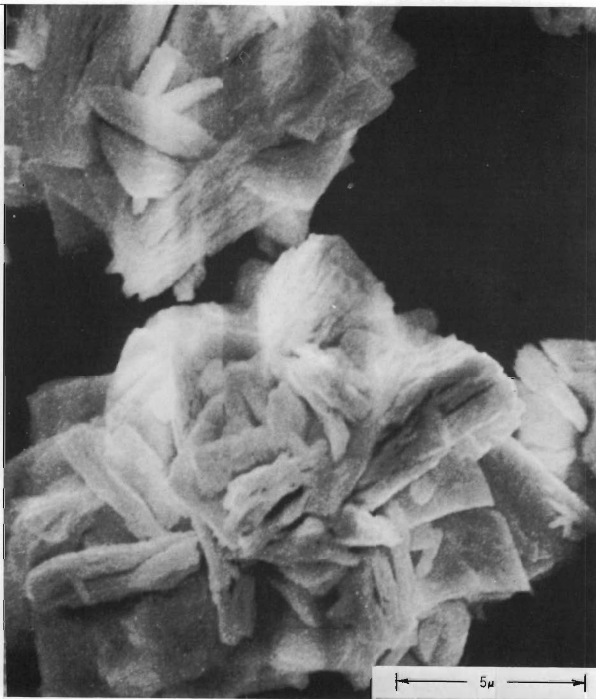
FIGURE 15. 450 °C CALCINED OXALATE SOURCE \text{PuO}_2 (10,000X)
