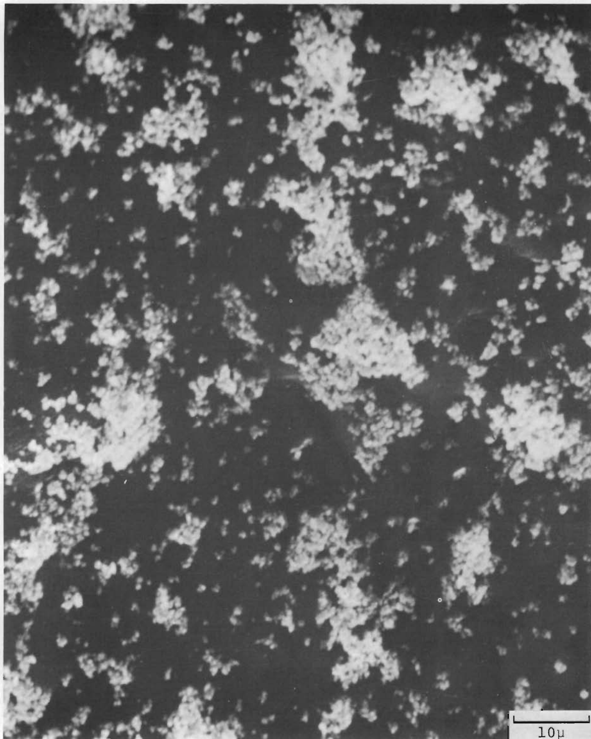
FIGURE 9. SCANNING ELECTRON MICROGRAPH OF 93% ENRICHED \text{UO}_2 (2000X)
