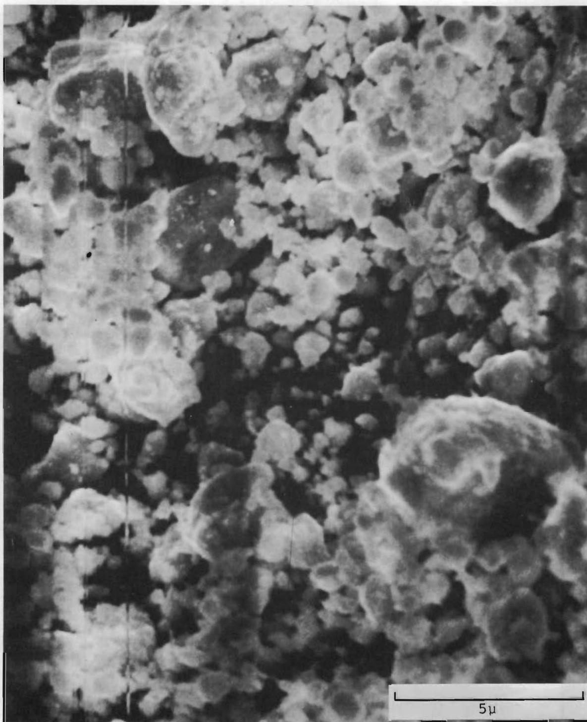
FIGURE 22. SCANNING ELECTRON MICROGRAPH OF 1000 °C CALCINED NITRATE SOURCE \text{PuO}_2 (10,000X)
