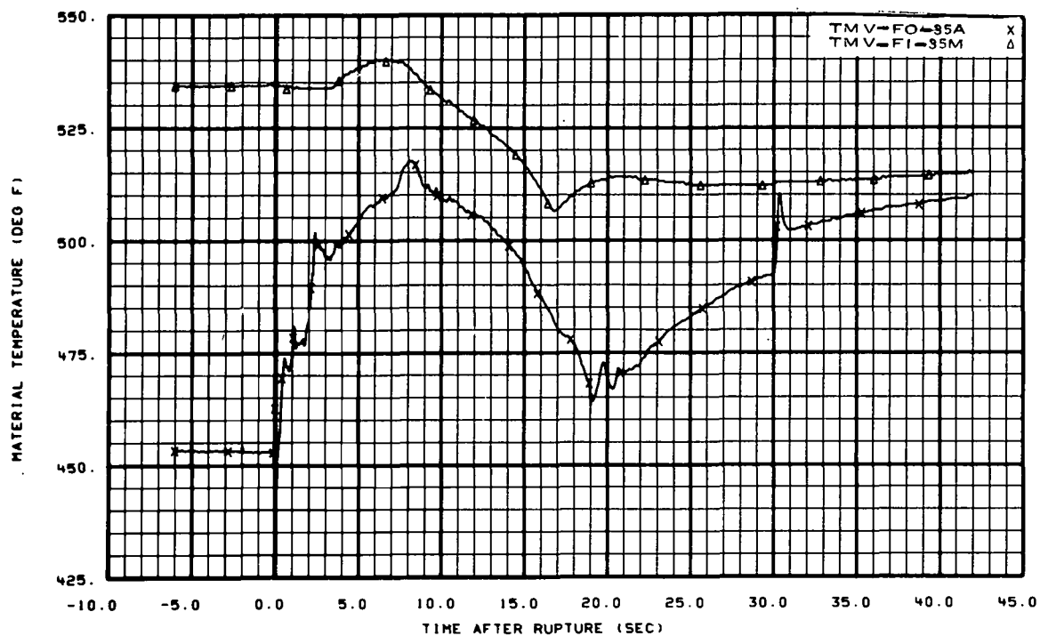
Fig. 25 Material temperature in vessel filler..
