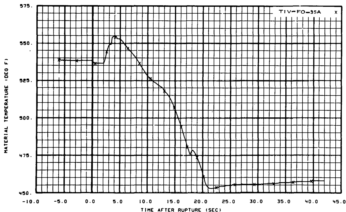
Fig. 26 Material temperature in vessel filler insulator.
