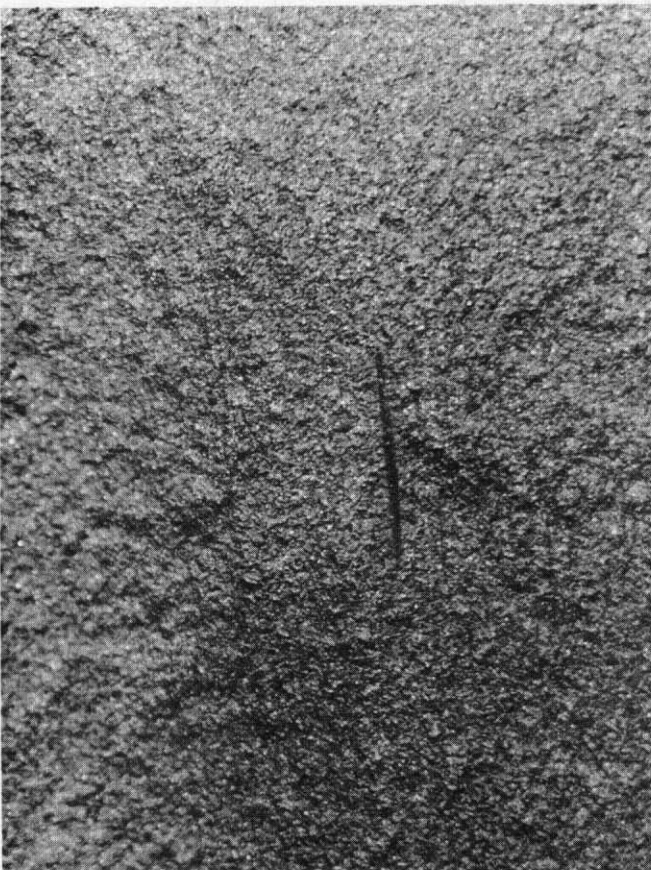
FIG. 17. EXAMPLES OF INCLUSIONS IN SPALLED RODS.
