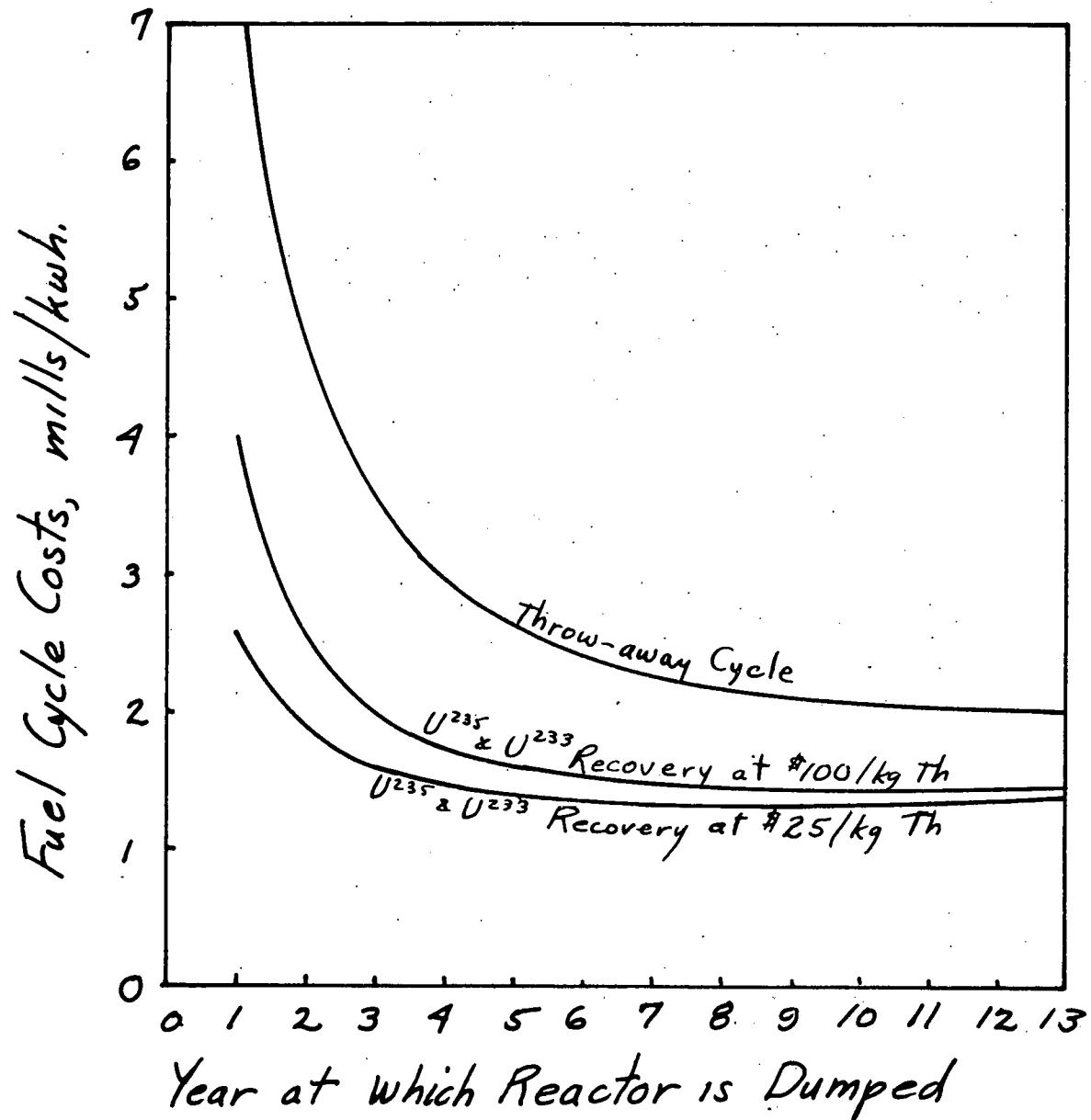
Fig. 3 Fuel Cycle Costs for 315 MWe Molten Salt Reactor
