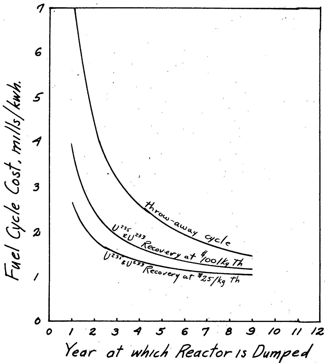
Fig. 7 Fuel Cycle Costs for 315 MWe Molten Salt Reactor with Continuous Fission Product Removal at Zero Cost
