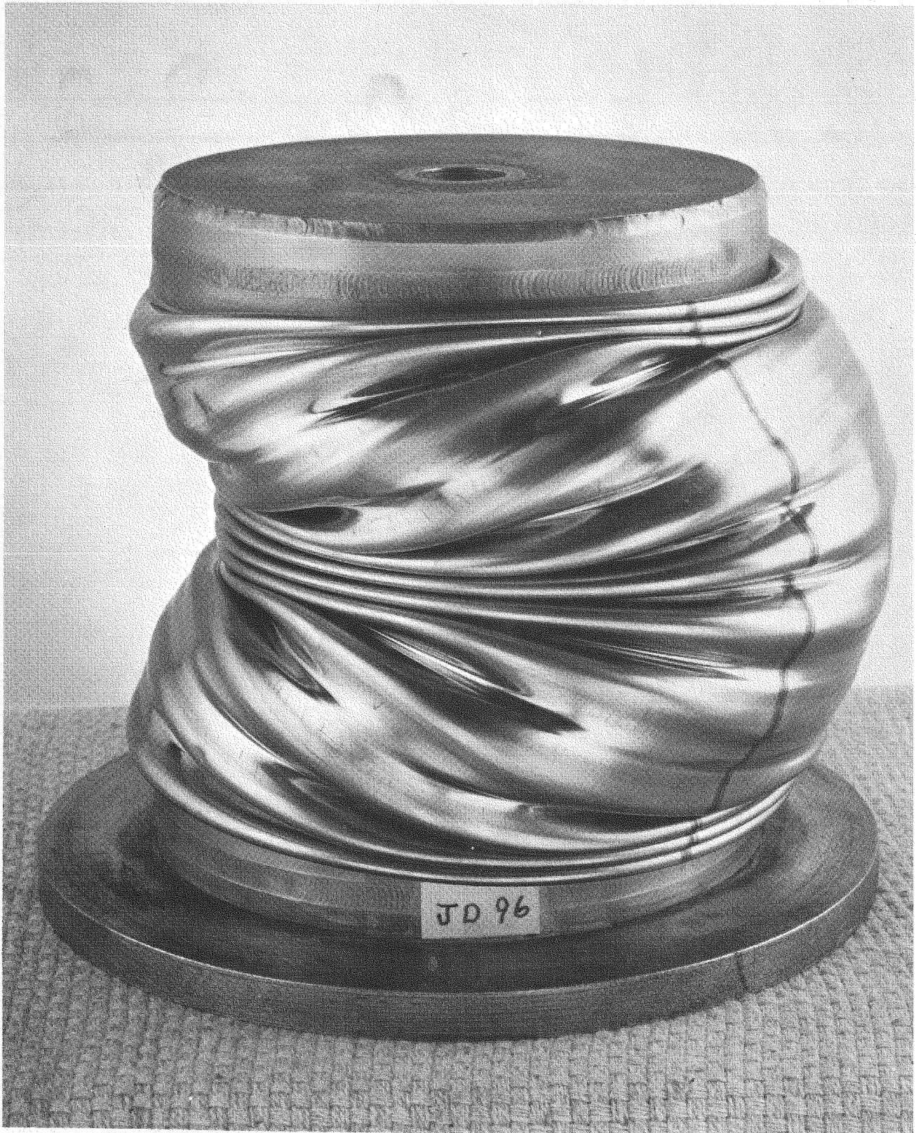
FIGURE 14.1. EXAMPLE OF SQUIRM IN BELLOWS, INTERNAL PRESSURE LOADING, ENDS FIXED
