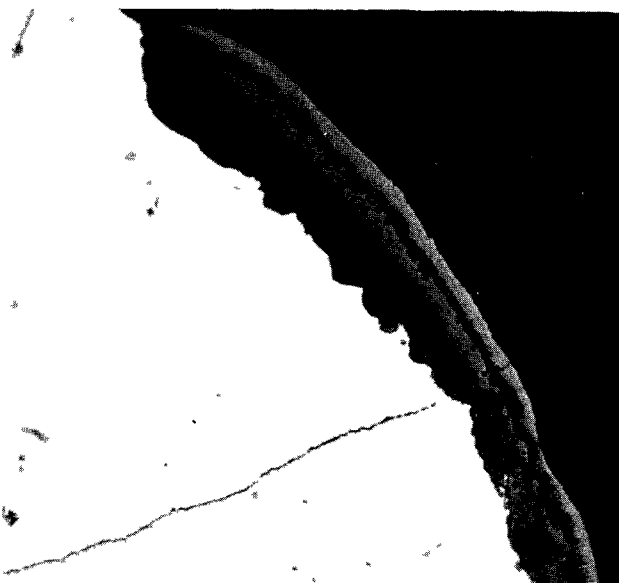
Fig. 14. Air oxidation of Incoloy 800. 600 X. Pretreatment: 1458 K, 10^{-5} torr, 1 h. Air exposure: 973 K, 0.78 atm, 8 h. Etch: Glyceregia, 90 s.
