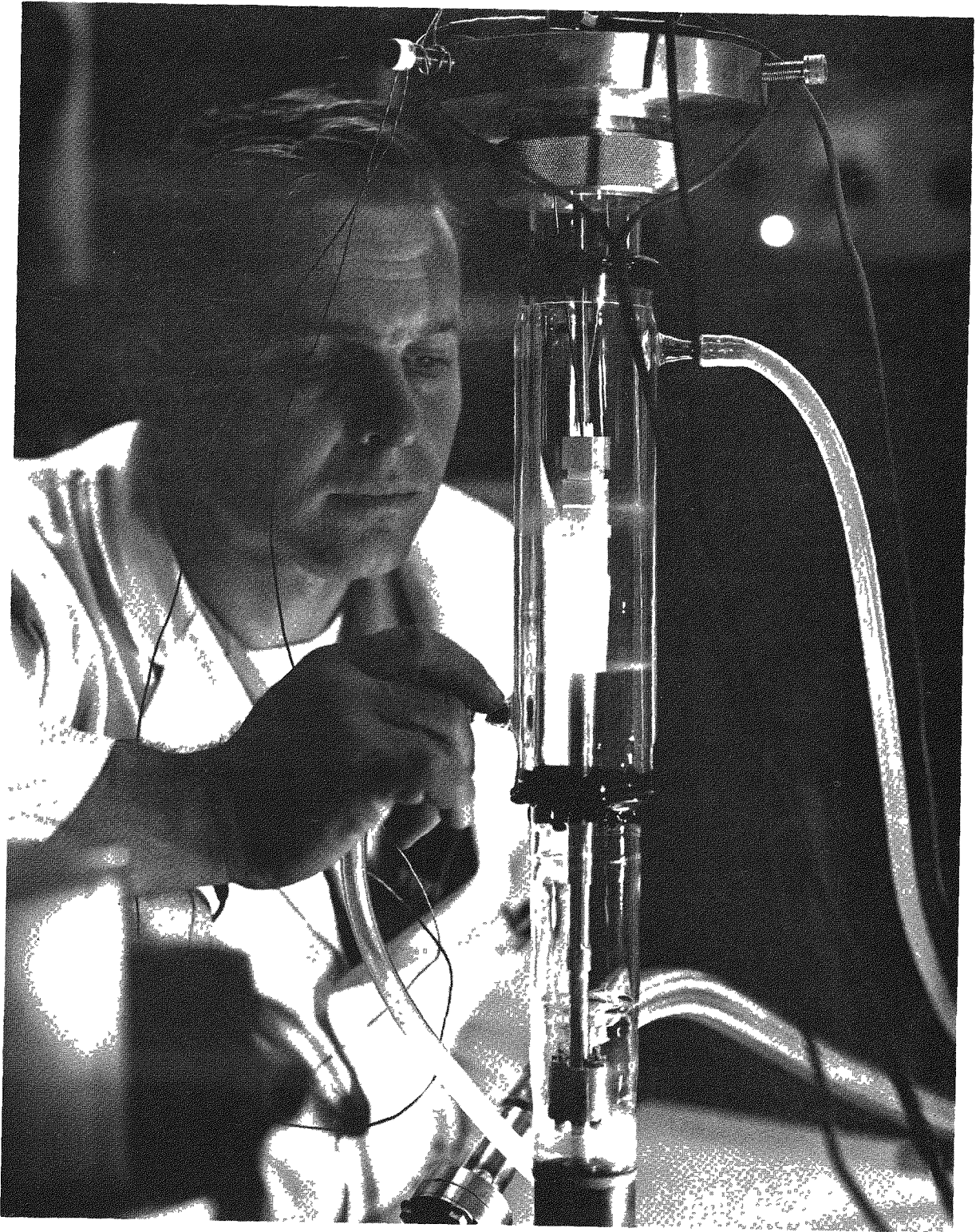
Fig. 3.10--Apparatus for final assembly and bakeout of Mark VI converters
