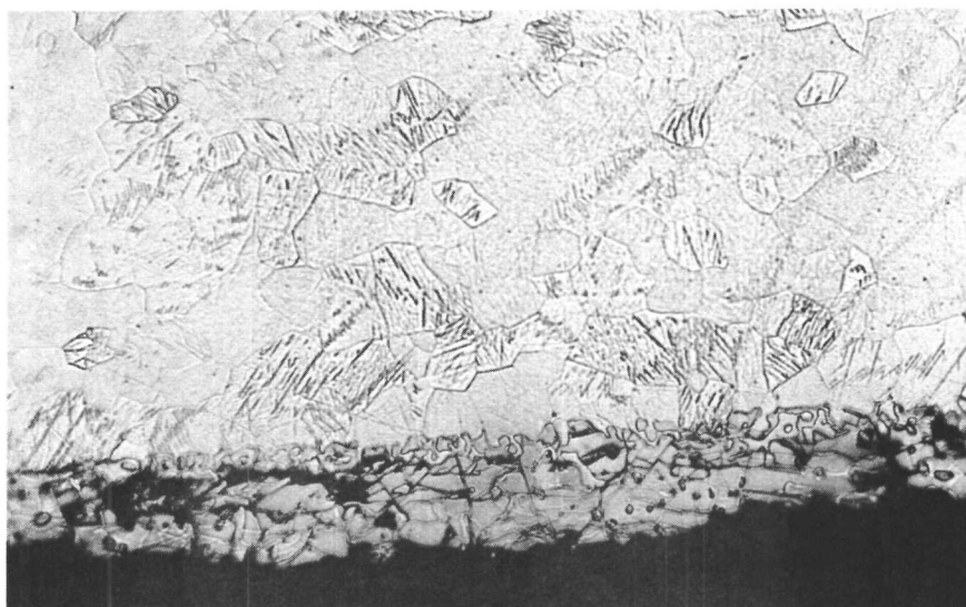
Fig. 2.10--Microstructures at the Re-UC interface of sample E 1
