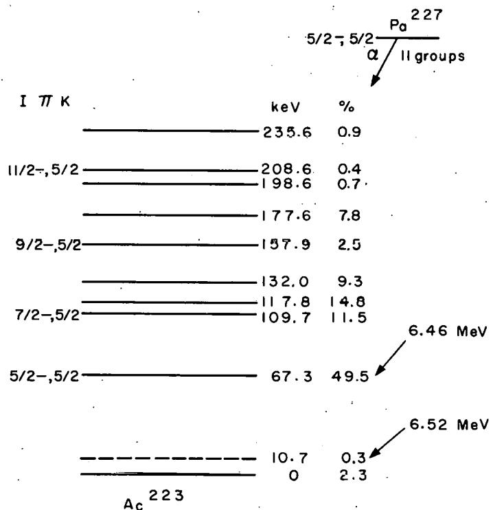
Fig. 5. Decay scheme of  $\text{Pa}^{227}$  (by Hill).
