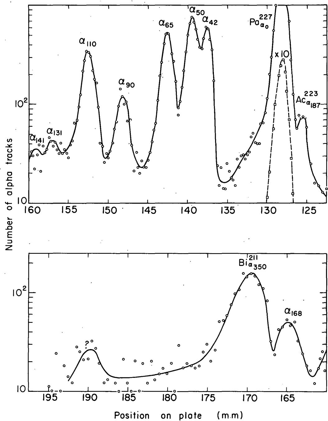
Fig. 4. Alpha spectrum of  $\text{Pa}^{227}$ .
