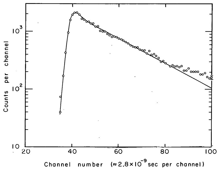
Fig. 27. Time delay between 300- and 27-keV  $\gamma$  rays of  $\text{Pa}^{231}$ .
