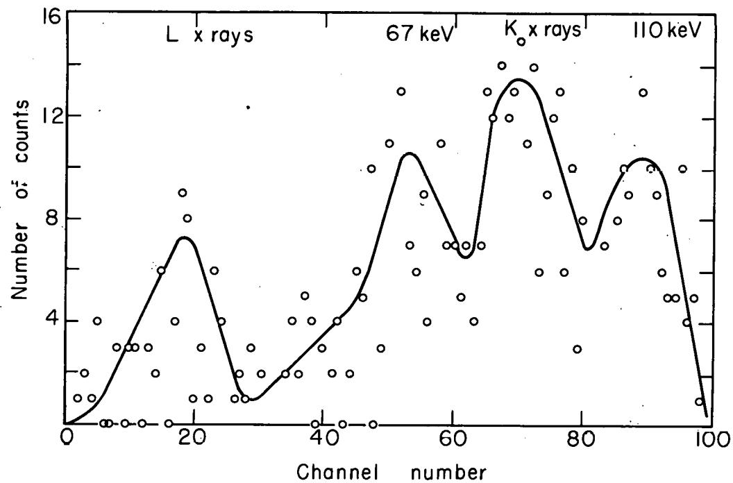
Fig. 7. Gamma spectrum in coincidence with  $\alpha_{110}$  of  $\text{Pa}^{227}$ .
