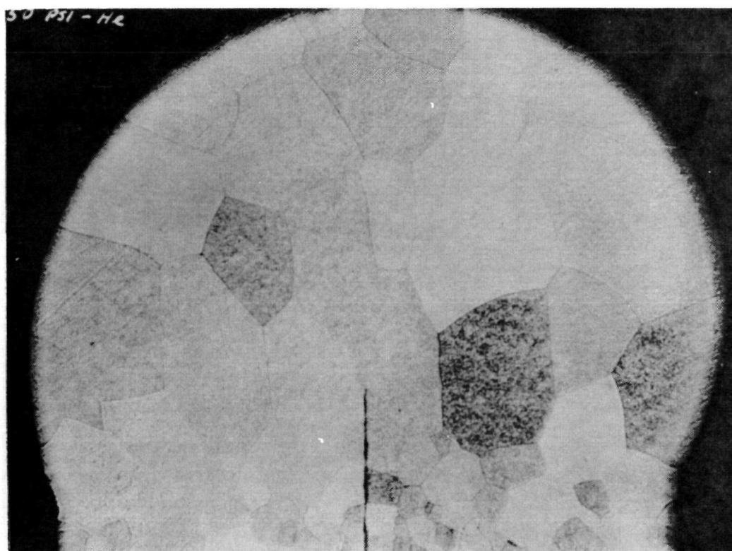
Fig. 44. Weld Zone of Molybdenum Disc R-3, Welded at 90 amps in 50 psi He--Magn 75X
