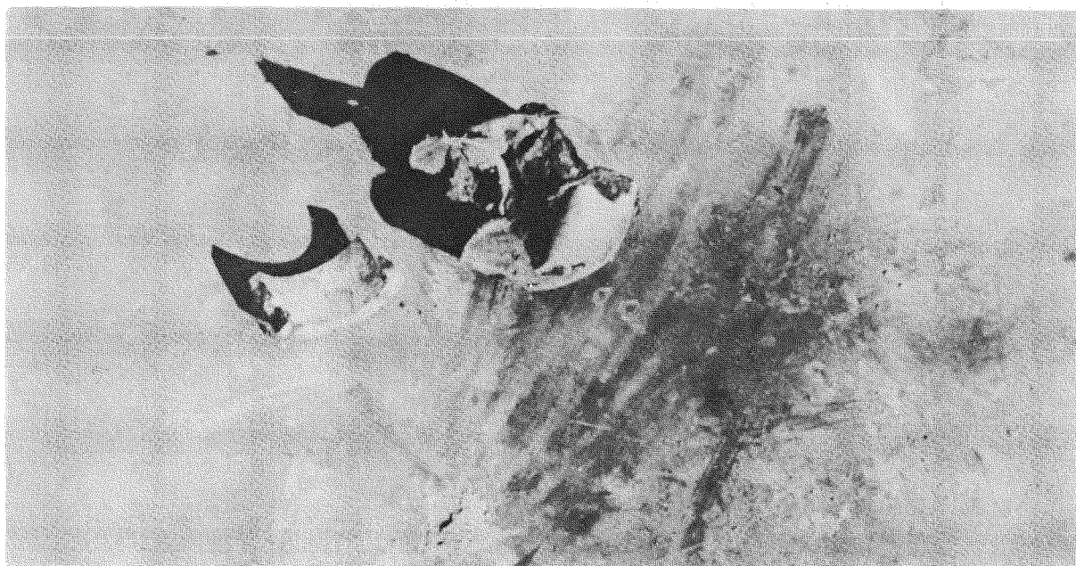
Fig. 62. View of Specimen 5 After Impact on Consolidated Rock Target
