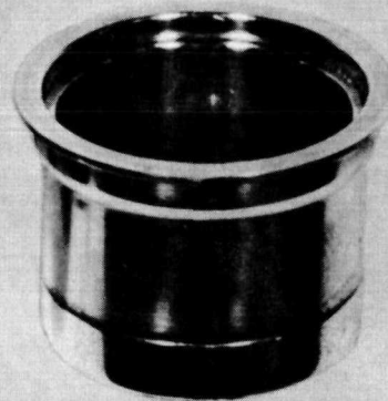
Sample 4-2 molybdenum + 0.5% titanium welded from rolled rod--unassembled.
