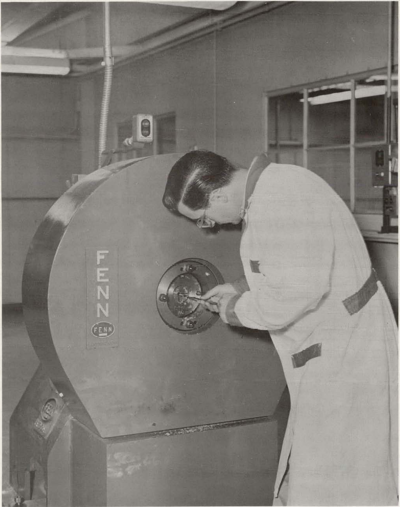
Figure 1.23 Swage-compacting of uranium dioxide power in 316L stainless steel tubes. (A-C Photo 210491).
