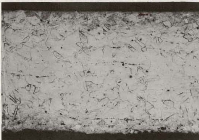
Figure 1.46 Swage-compacted alumina-filled fuel-rod cladding reduced from 0.325 to 0.250 to 0.225 in. o.d. (54.1 per cent) and straightened in 5-roll (left) and 6-roll (right) rotary straighteners. Top to bottom: transverse 50X, transverse 150X, and longitudinal 150X. (NP Photos 24A-3-2, -1, -3 (left); and 24A-9-2, -1, and -3 (right)).
