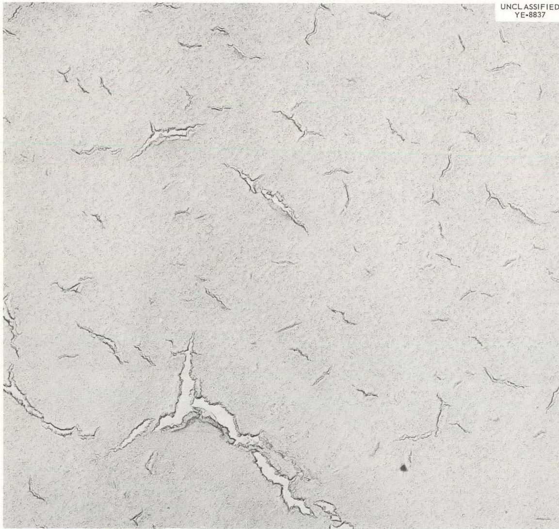
Fig. 18. Replica of Titanium Film Prepared by 1-hr Evaporation in High Vacuum at Liquid-Nitrogen Temperature. 7,500X. Reduced 20%.
