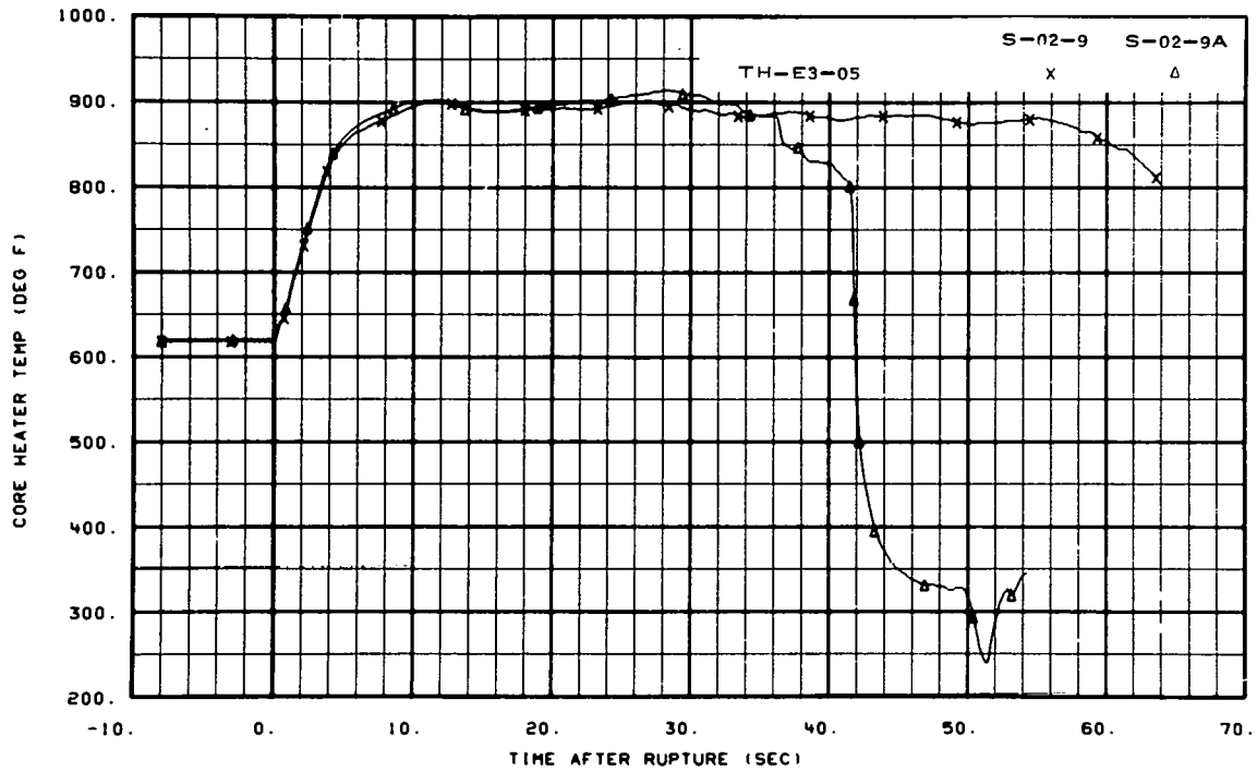
Fig. 99 Core heater temperature, Rod E-3 (TH-E3-05).
