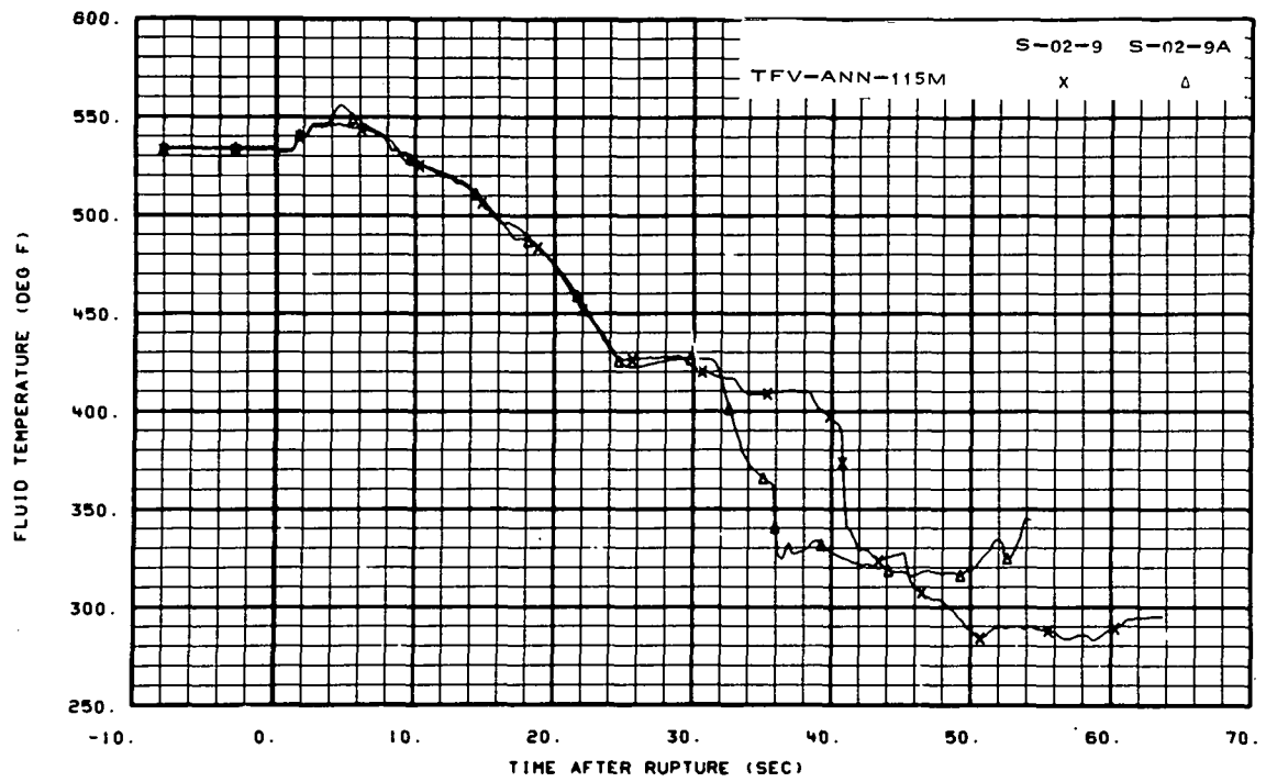
Fig. 21 Fluid temperature in downcomer annulus (TFV-ANN-115M).
