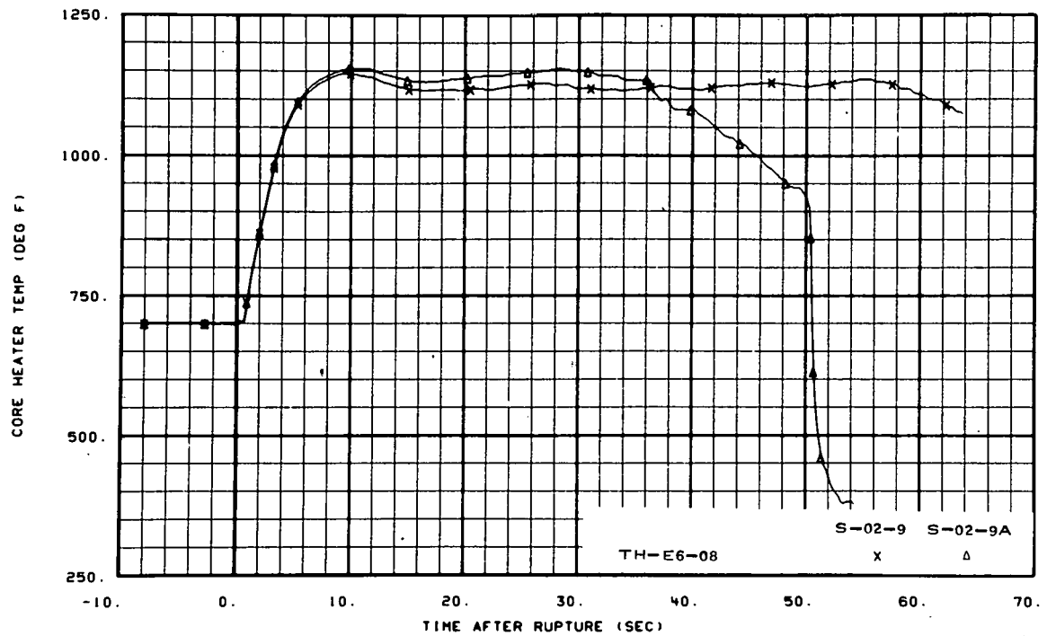
Fig. 101 Core heater temperature, Rod E-6 (TH-E6-08).
