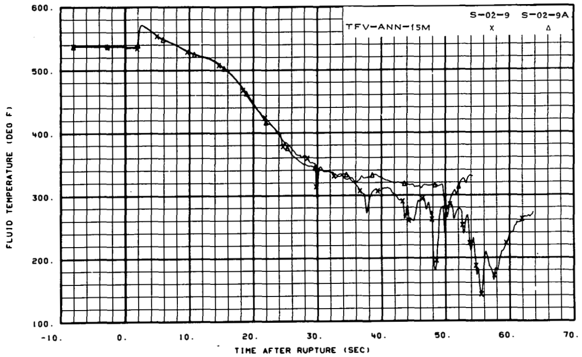
Fig. 17 Fluid temperature in downcomer annulus (TFV-ANN-15M).
