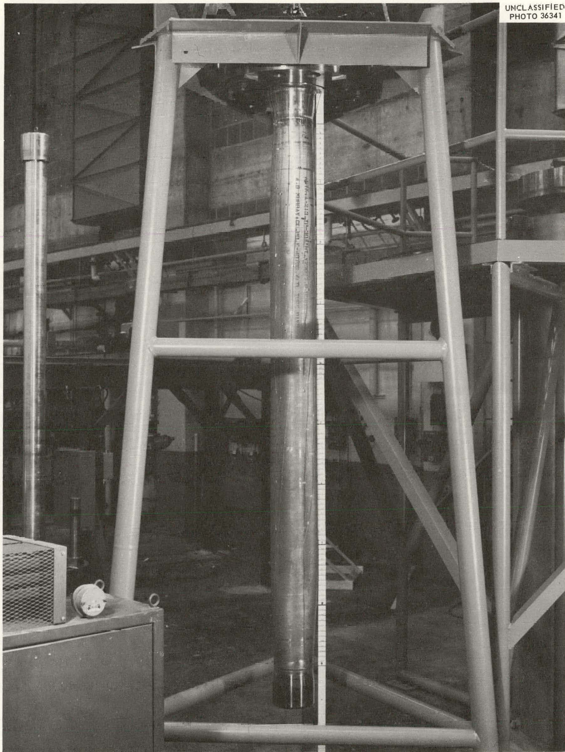
Fig. 2. Collapsed 8.0-in.-OD, 0.25-in.-Wall Type 304 Stainless Steel Specimen RD-1.
