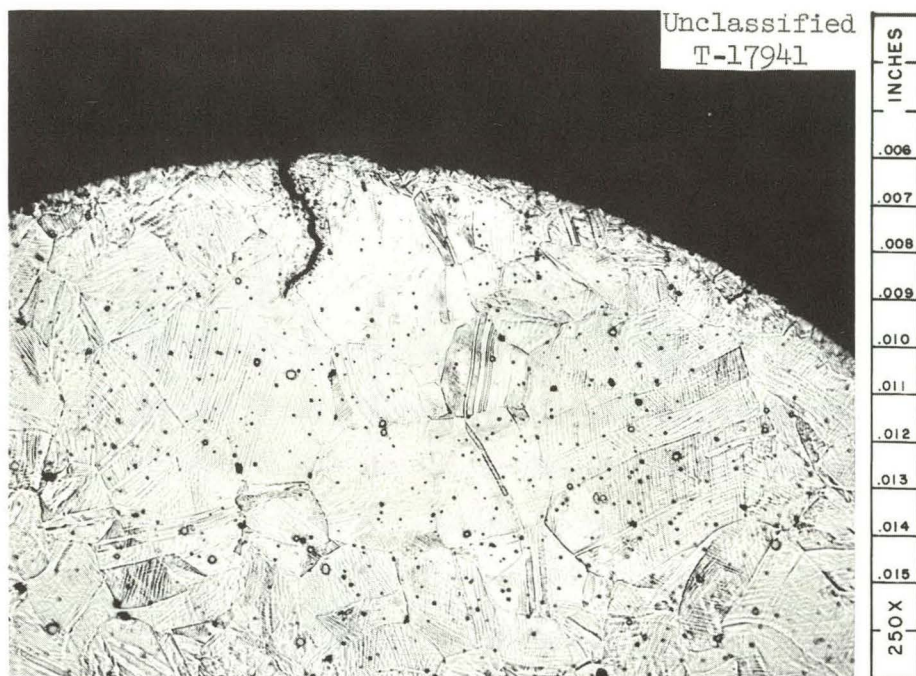
Fig. 12. As-Received Microstructure of Hastelloy W Spacer Wires. Etchant: 3 parts HCl, 2 parts H 2 O, 1 part 10% Chromic acid. 250X
