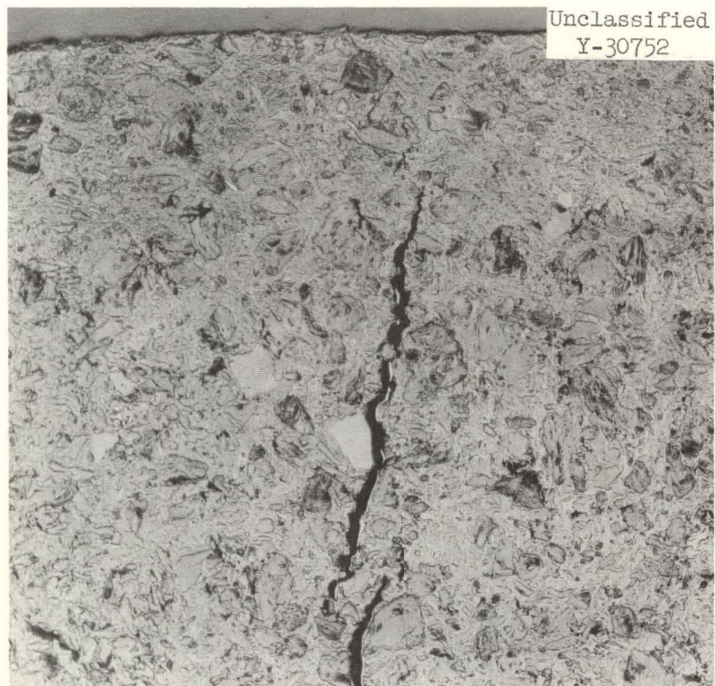
Fig. 7. Low Permeability Graphite: Typical Microstructure of 1/2-in.-diam Rods (a) As-Received and (b) After a One-Year Exposure to \text{LiF-BeF}_2\text{-UF}_4 (62-37-1 mole %). As polished. 100X
