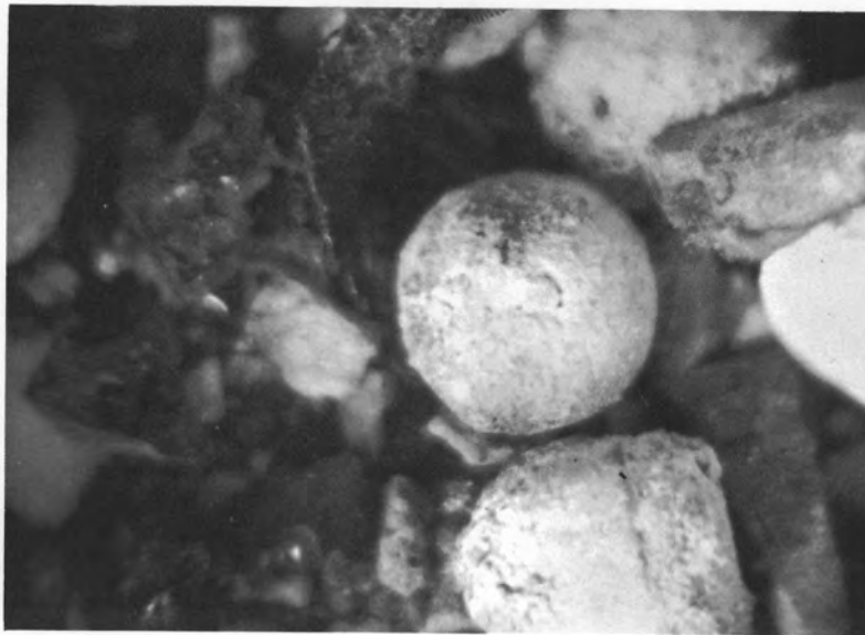
Fig. 11.2. Black Vitreous Material Recovered from Thoria-Pellet Irradiation Experiment C-43-3.
