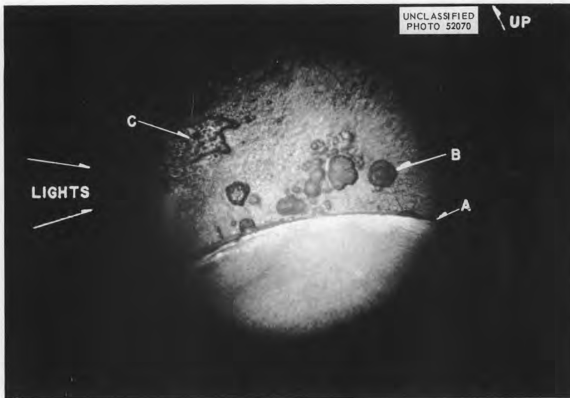
Fig. 1.9. Mound Deposit at Top of Upper Patch. (A) Top edge of upper patch. (B) and (C) Mound deposits. Location: top center of upper patch. 4X. Reduced 6%.
