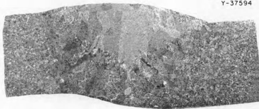
Fig. 15.8. Completed Weld in Zircaloy-2 with a Misalignment of 0.075 in. Etchant: \text{H}_2\text{O} , \text{HNO}_3 , \text{HCl} , \text{HF} solution. 4X.
