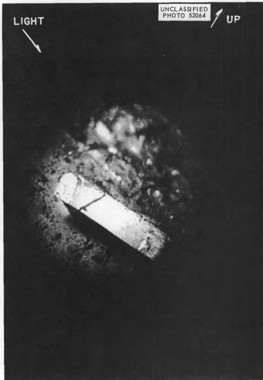
Fig. 1.7. Y-Fracture Screen Stub, Screen 5. Location: on stub line on top of lower patch, about 10 to 15° east of building north. Point of focus is the fracture face. Black deposit is \text{WO}_2 . See Fig. 1.8. 4X.
