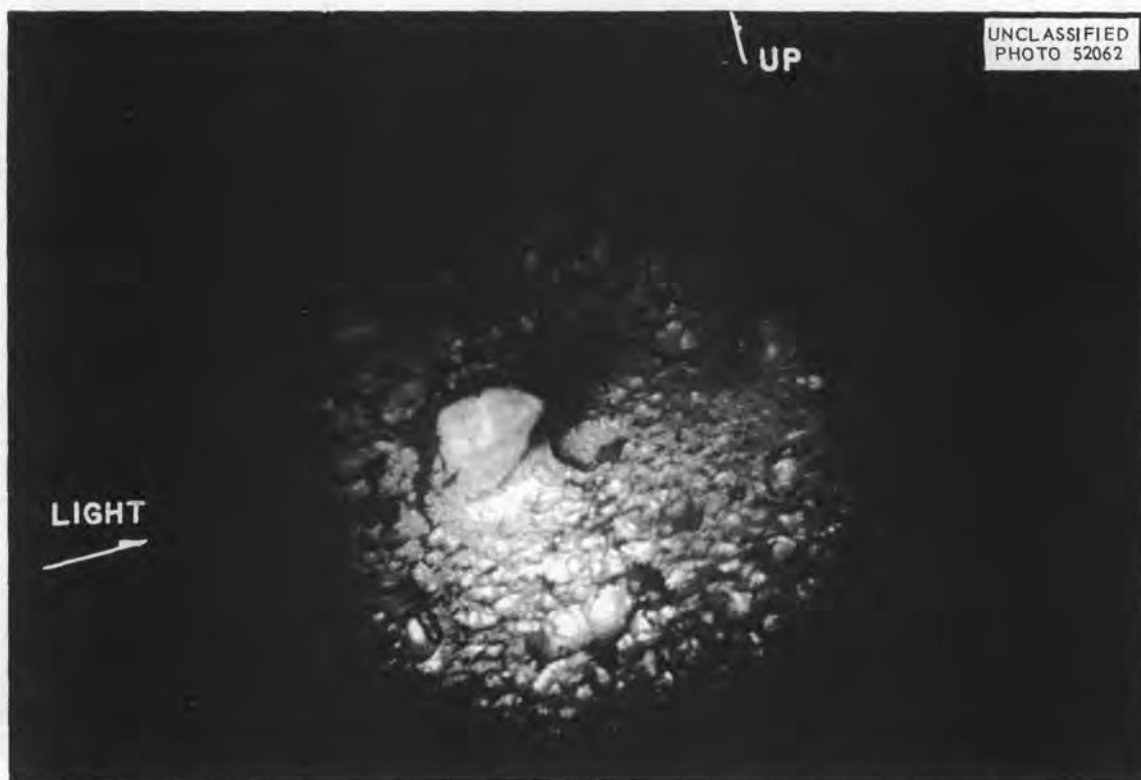
Fig. 1.5. Screen Stub and Pit Region at Screen 4. Location: fourth screen from top and about 5° west of building north. Black deposits are WO_2 from broken light bulb filaments. See Fig. 1.6. 4X. Reduced 8%.
