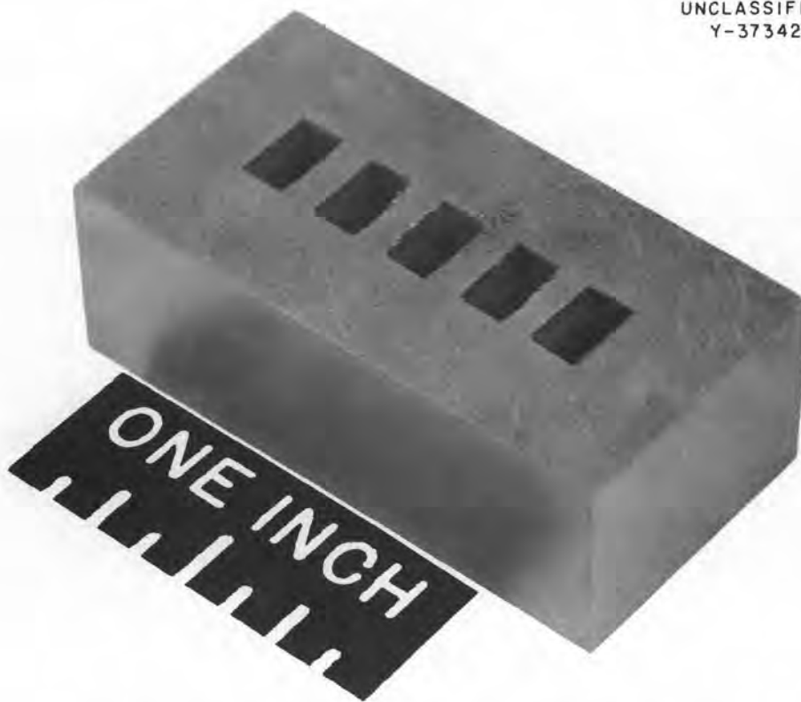
Fig. 15.2. Zircaloy-2 Specimen Milled by Spark-Discharge Machining.
