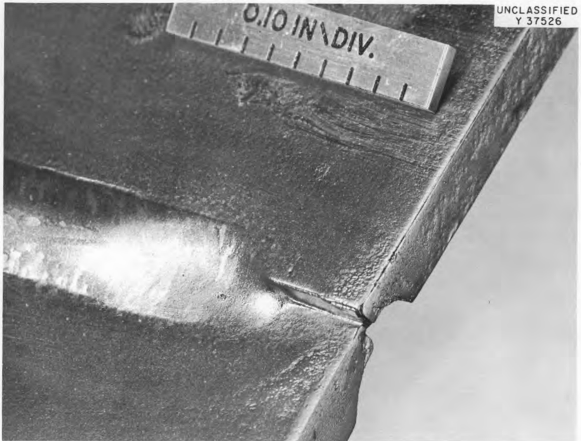
Fig. 15.6. Root Pass with Plate Misalignment of 0.090 in.
