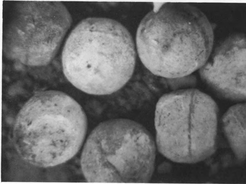
Fig. 11.1. Irradiated Thoria Pellets.
