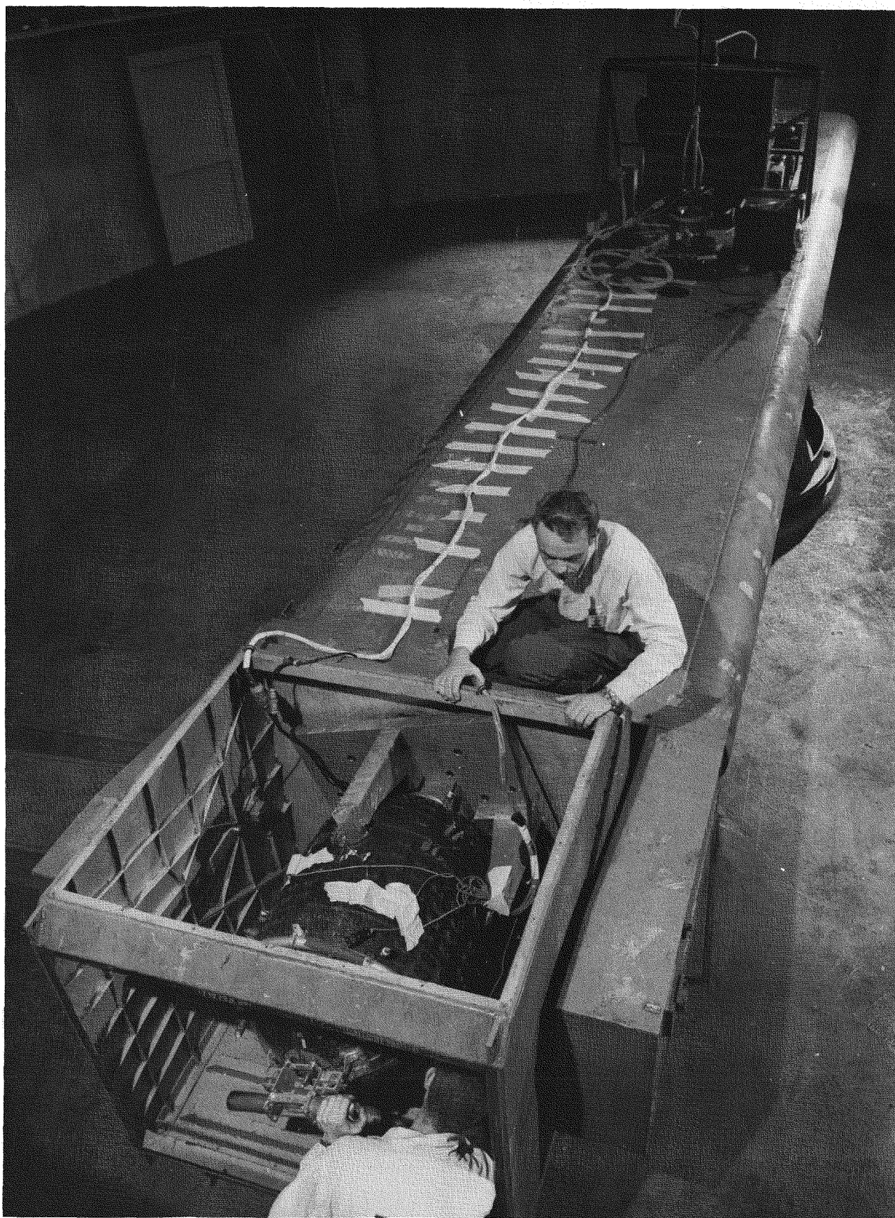
Fig. II-3. SNAP IA G-2 Generator--Vertical Acceleration Test Arrangement
