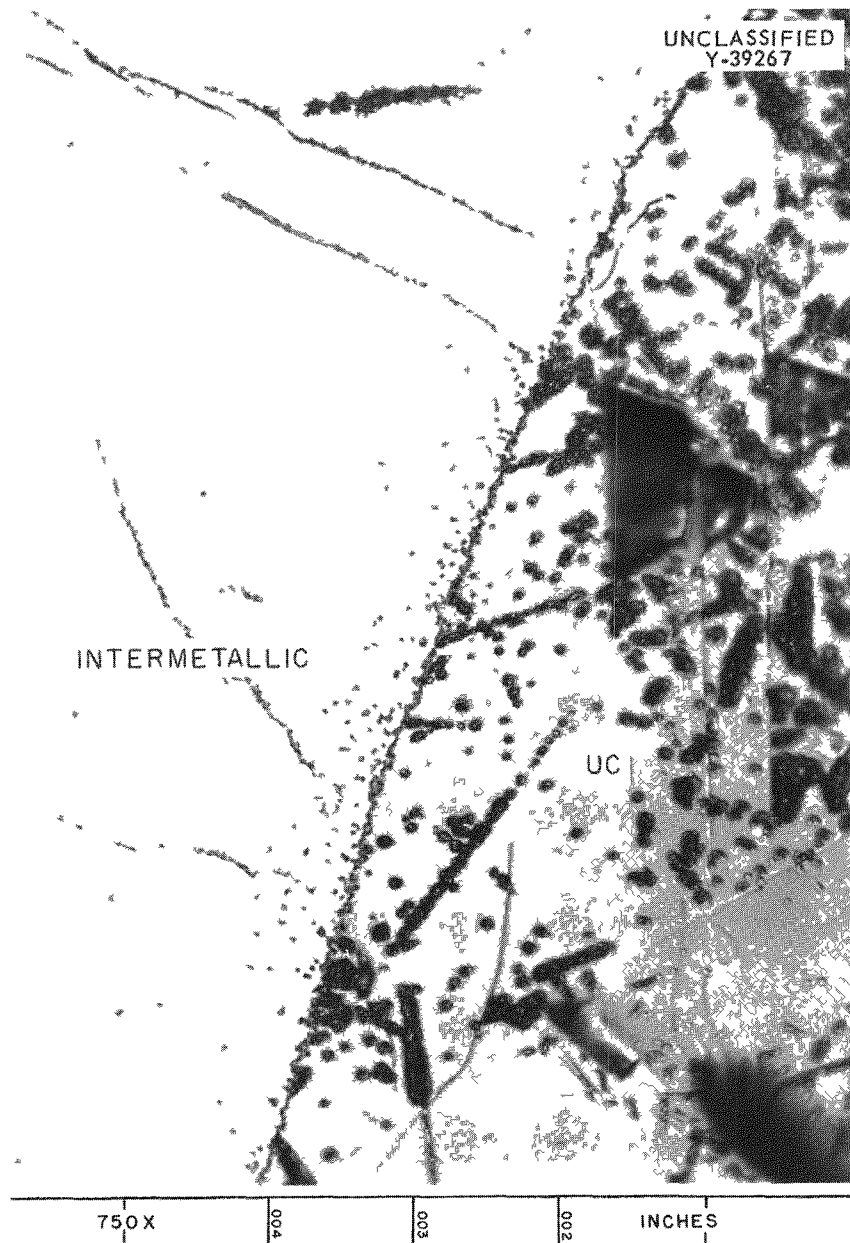
Fig. 4.8. Interface Between UC and Intermetallic Phase. Note the finely dispersed precipitate within the intermetallic matrix.
