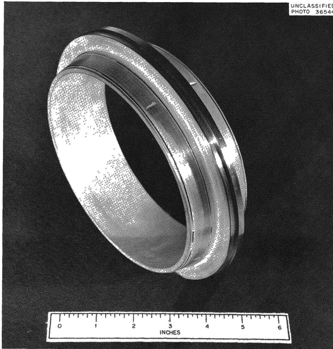
Fig. 7.12. Sample 6-in.-IPS Double-Seal "Grayloc" Modified Seal Ring.
