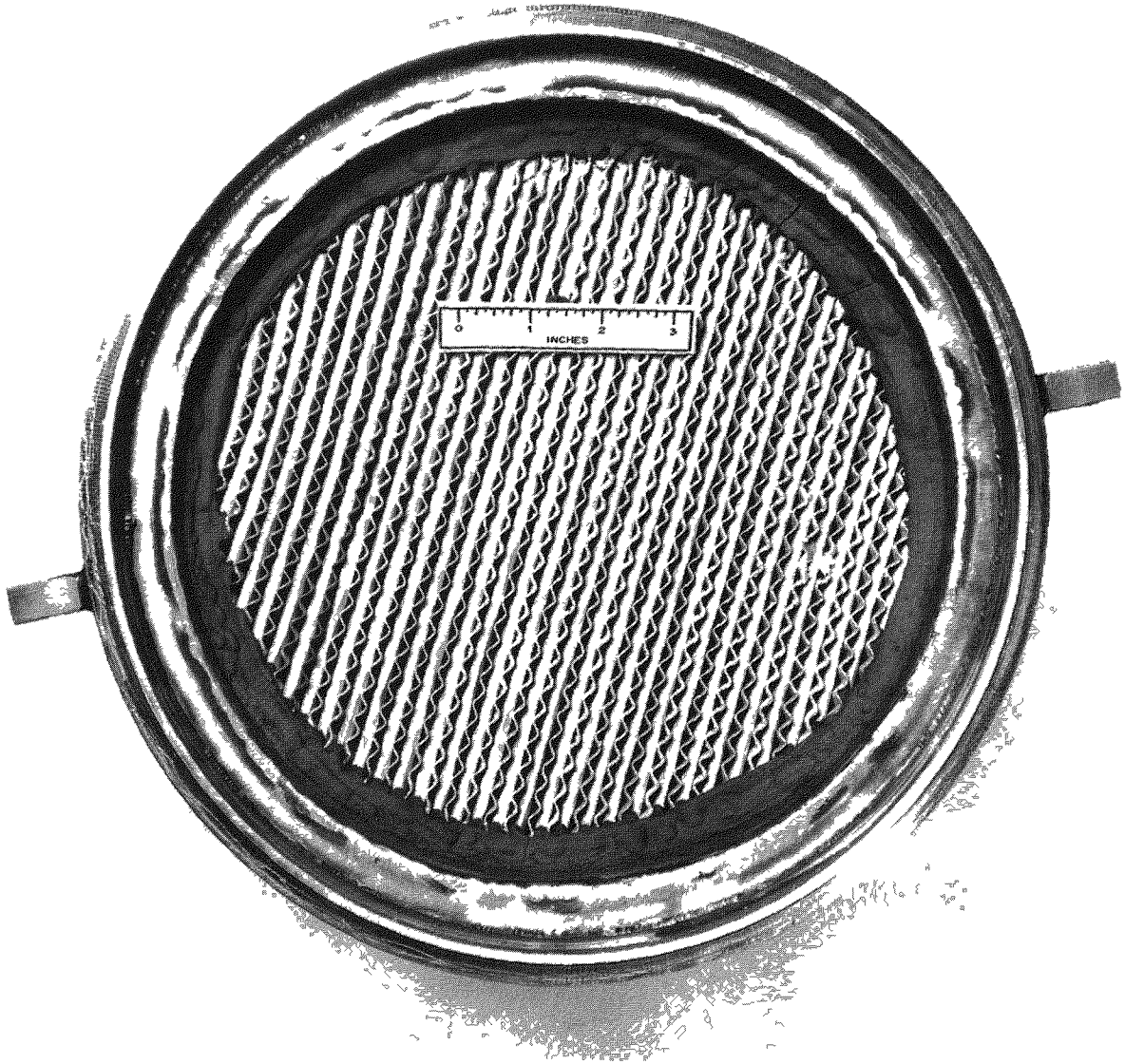
Fig. 7.19. Filter Unit No. 2 After Thermal Cycling and Efficiency Tests.
