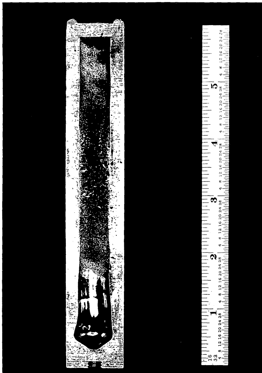
Figure 4. - Section through molybdenum reflux capsule exposed to boiling, splashing cesium at 2500 F for 54\frac{1}{2} hours. Effect may be due to Redox reaction involving a volatile molybdenum oxide or merely to hot cesium solution splashing against a cooler wall and precipitating dissolved molybdenum.
