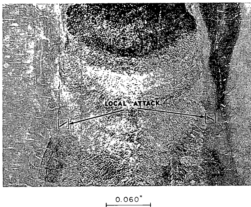
Figure 7. - Localized attack observed on the surface of a Cb-1Zr weld exposed to liquid potassium for 1000 hours at 2000 0 F.
