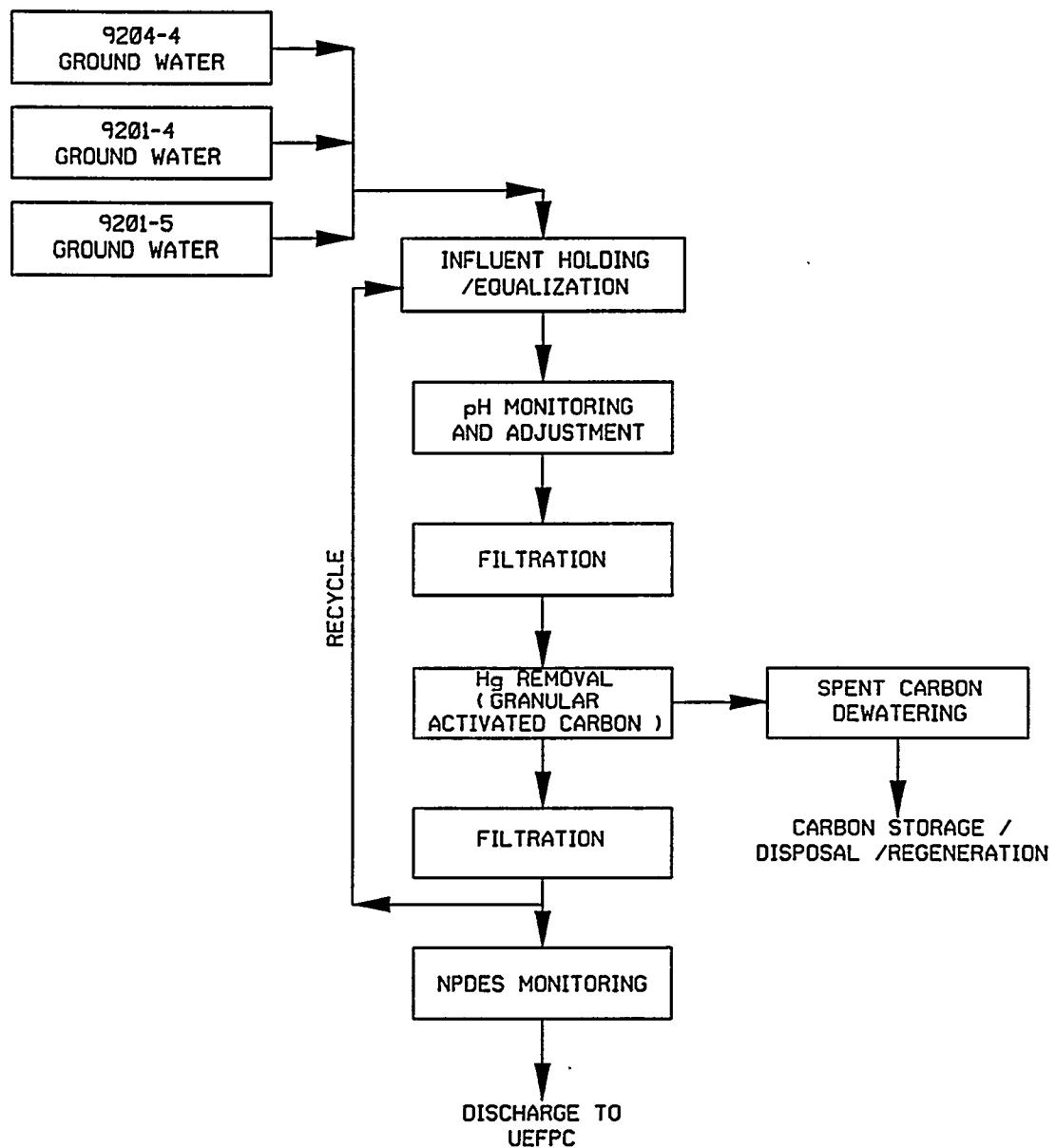
FIG. 3 : BLOCK FLOW DIAGRAM
