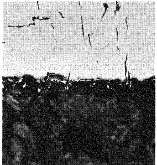
Figure 48. Graphite-Mo interface showing possible reaction layer. 400 \times , unetched.
