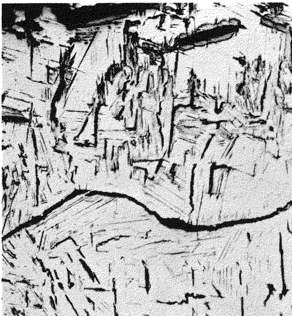
Figure 47. Mo-C alloy formed at Mo-brazed graphite joint. Estimated C, 7 to 10%. 250 \times , unetched.
