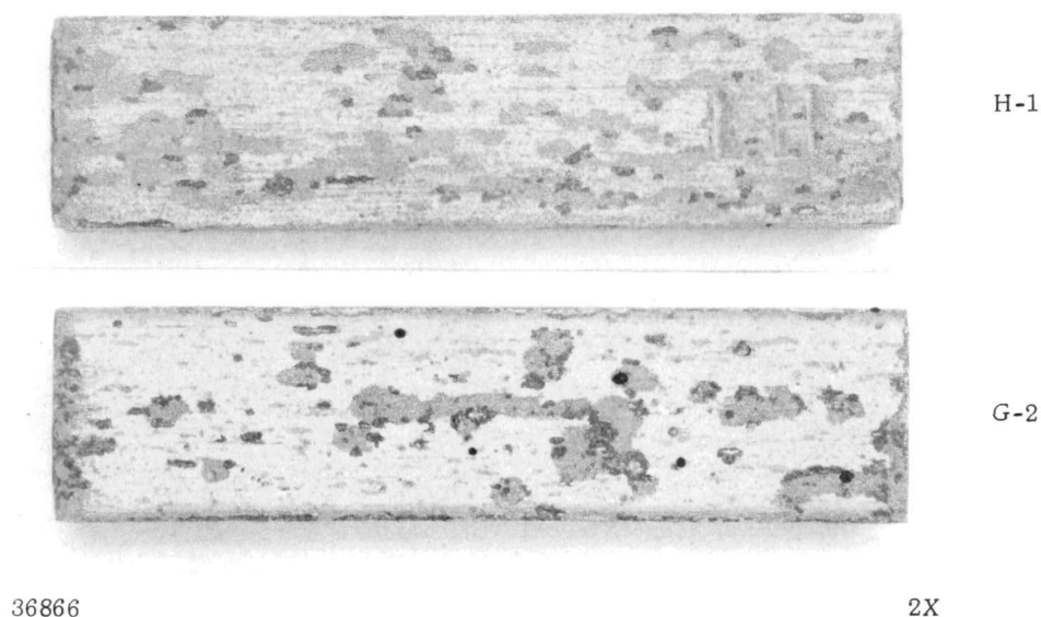
Figure 16. Trefimetaux Corrosion Specimens after 89 Days in 315°C Water Flowing at 5.5 m/second
