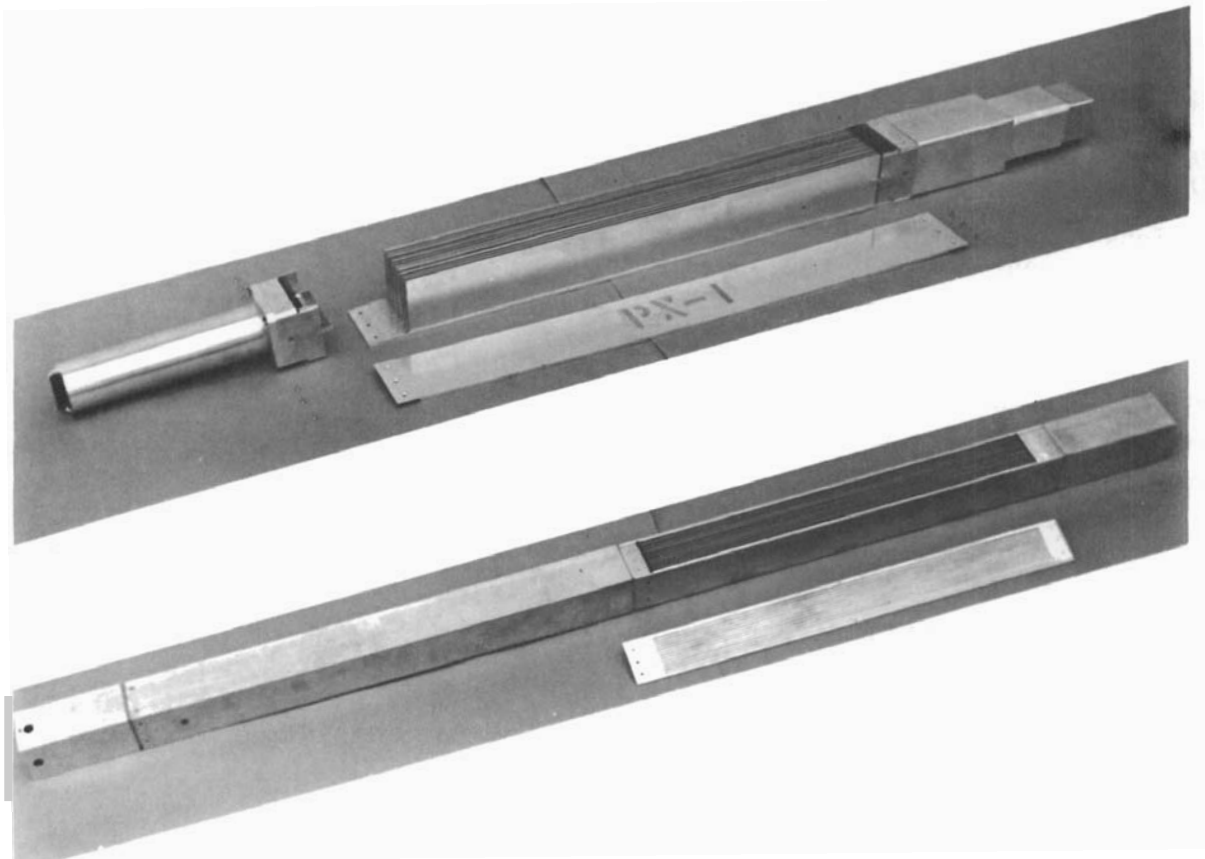
FIGURE 4. PRCF- Phoenix Core. Shim Rod with Fuel Follower and Stationary or Fixed Assembly
