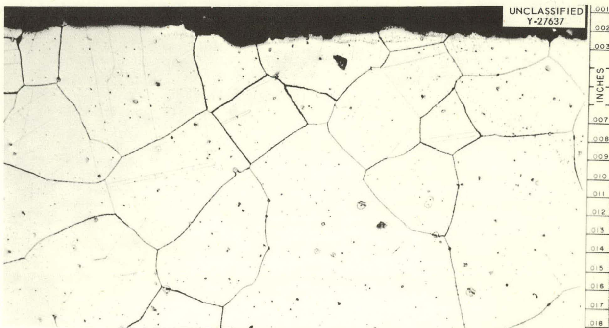
Fig. 77B. Portion of Fig. 77A. Typical Surface and Microstructure, Etchant: Aqua regia. 200X.
