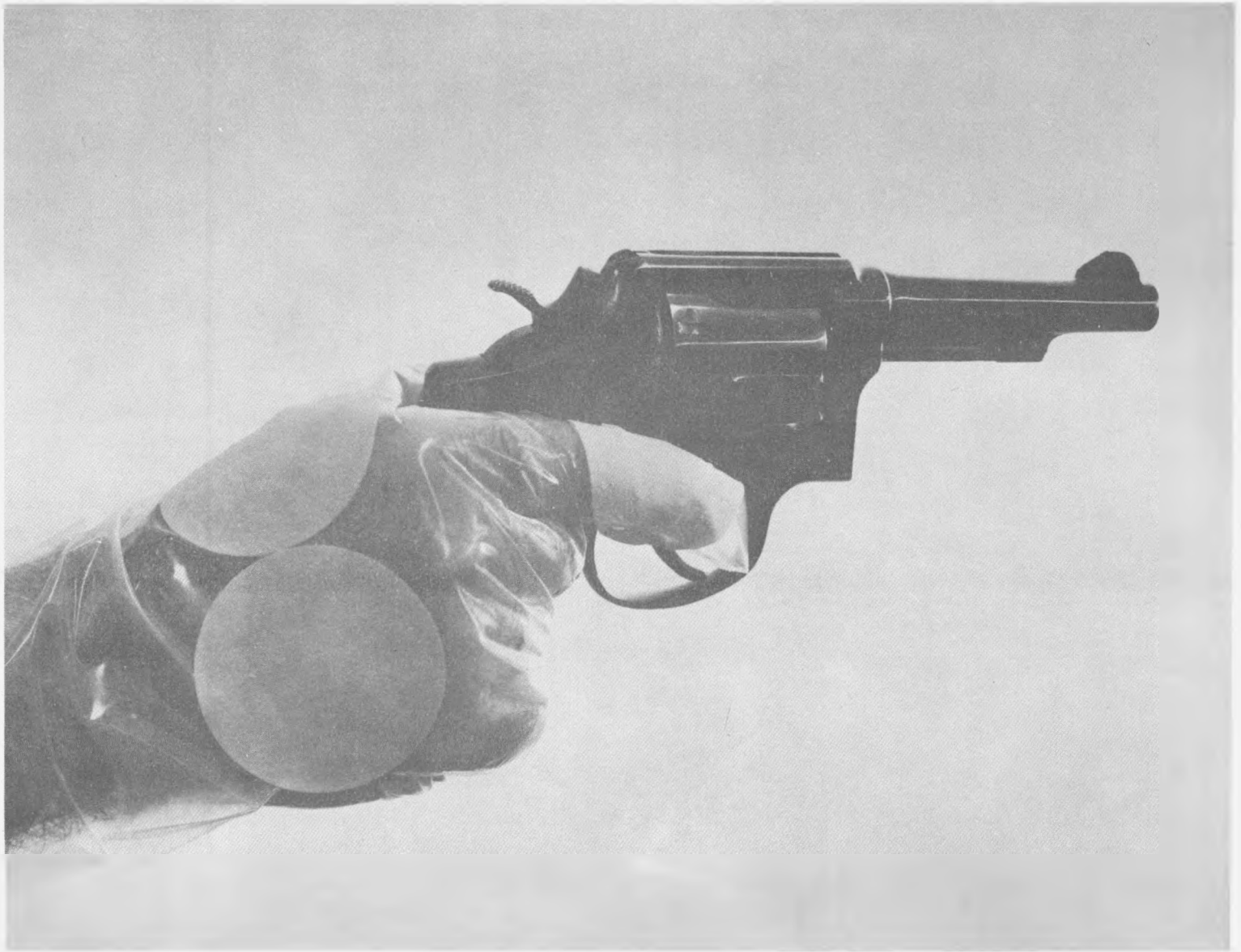
Fig. 9. Plastic glove with moist filter paper patches for gunshot-residue distribution studies
