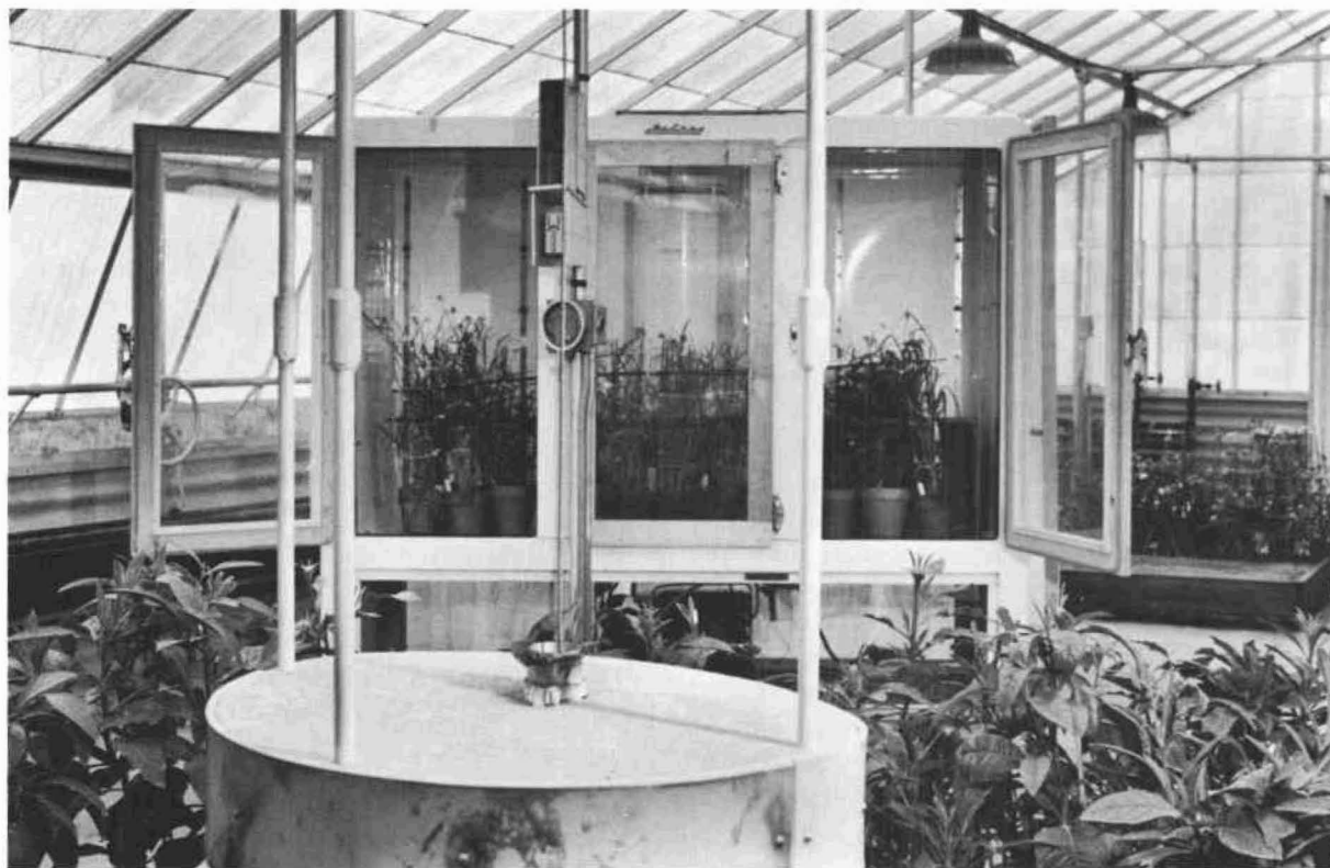
Figure 4. Facility for irradiation of plants under controlled environmental conditions. The chamber in the background provides for growth under prescribed conditions of illumination, temperature, and humidity. A radioactive cobalt source is housed within the lead shield in the foreground.
