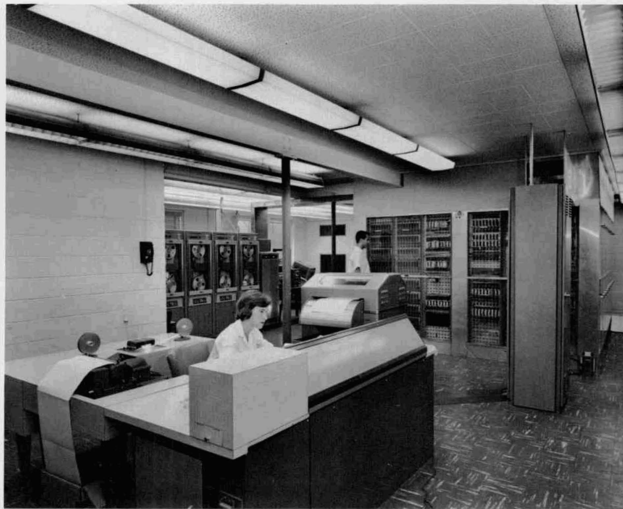
Figure 1. View of the high-speed digital computer Merlin, designed and constructed at Brookhaven. In the foreground are the high-speed printer and manual control console. The vertical racks to the right rear constitute part of the control section.
