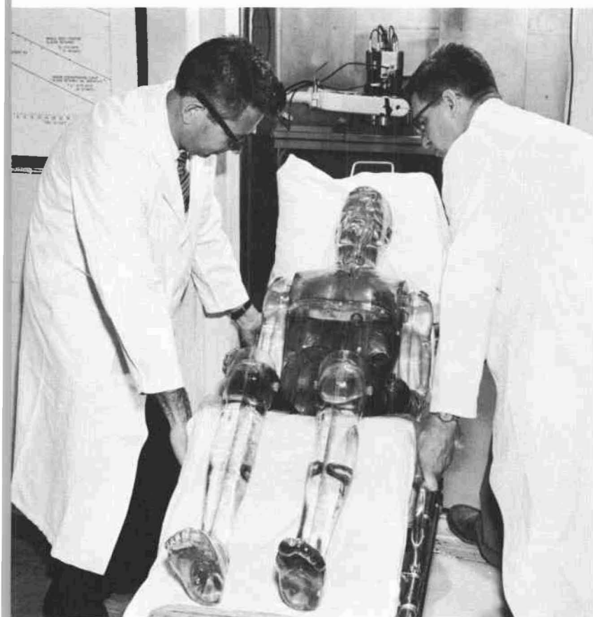
Figure 5 (Top, left). Plastic phantom, placed in standard measuring position, is positioned under a detecting crystal of thallium-activated sodium iodide.
