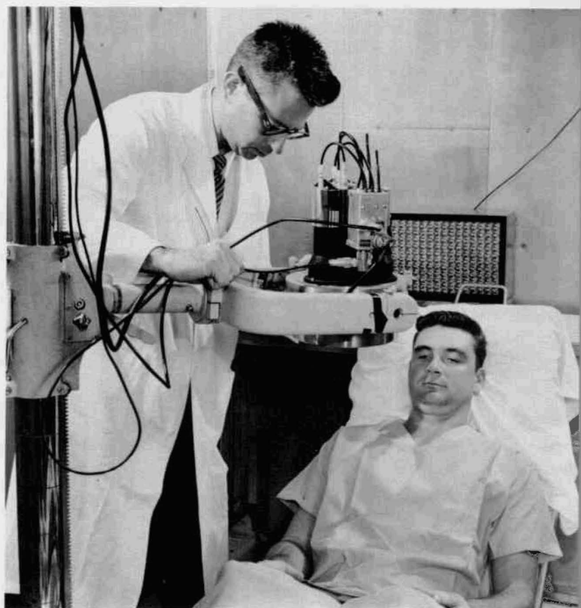
Figure 10. Crystal detector is positioned over a patient from the Industrial Medicine Clinic who may have been exposed to internal radioactive contamination. By whole-body measurement, the presence and extent of such contamination can be determined.
