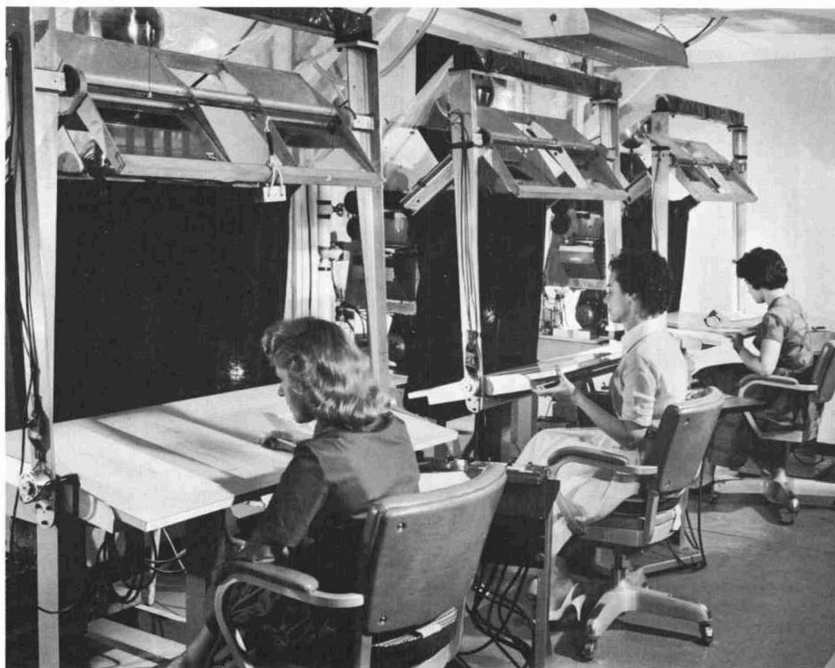
Figure 13. Bubble chamber film is given careful inspection for all nuclear interactions of interest to physicists. These machines, known as scanning tables, project an image of the bubble chamber film enlarged to actual size, so that each frame may be inspected easily. Scanning is the first in a series of operations designed to extract information from the film.
