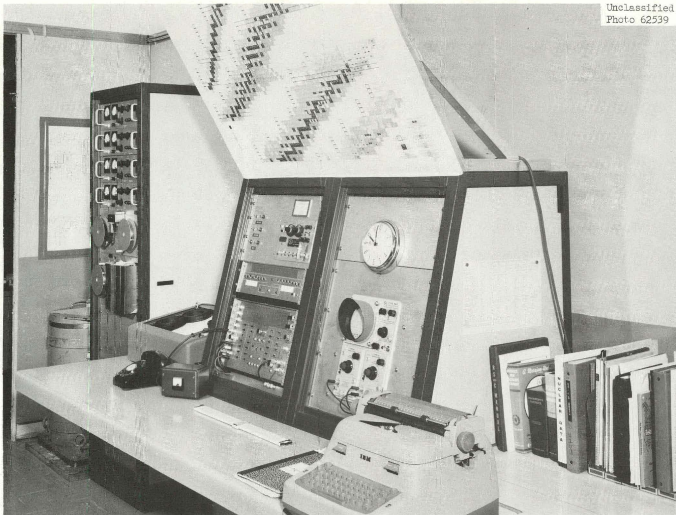
Fig. 17. Gamma-Ray Spectrometer for Loop and Capsule Experiments. Installation for analysis of fission products, argon activation, and corrosion products as applicable to ORR poolside and eight-ball capsules, ORR loop No. 1, ORR loop No. 2, and pressurized-water loop.
