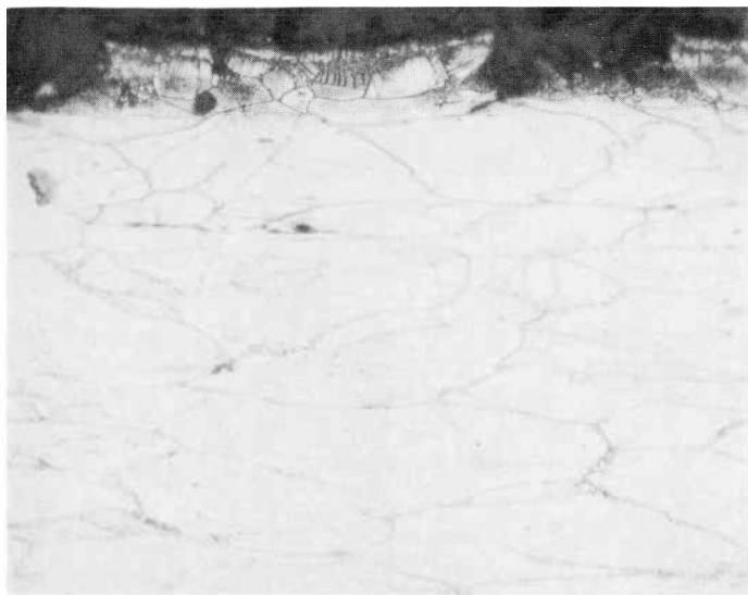
FIG. 39 - PRE-EXPOSED 316 ss CREEP RUPTURE IN SODIUM Rupture Time - 903 hrs
