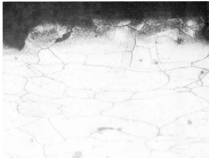
FIG. 38 - PRE-EXPOSED 316 ss CREEP RUPTURE IN SODIUM Rupture Time - 632 hrs
