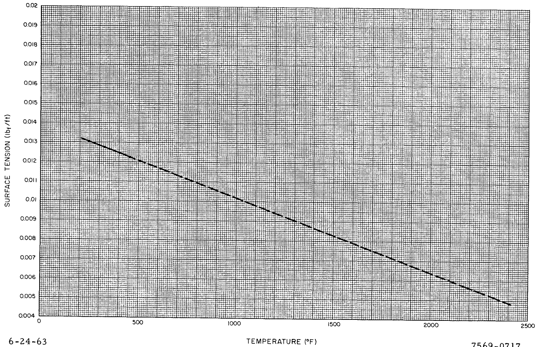
Figure 1.36 Surface Tension of Sodium (Liquid) (Reference 19)
