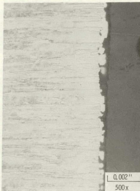
(b) High Purity ^{90}\text{SrF}_2 1100°C, 4400 Hours
