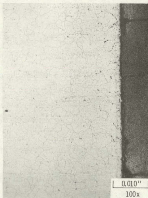
(c) High Purity ^{90}\text{SrF}_2 1000°C, 4400 Hours
