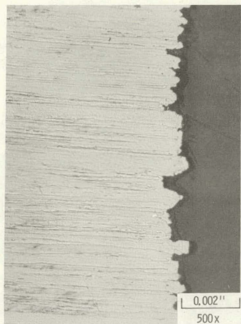
(a) High Purity ^{90}\text{SrF}_2 800°C, 4400 Hours
