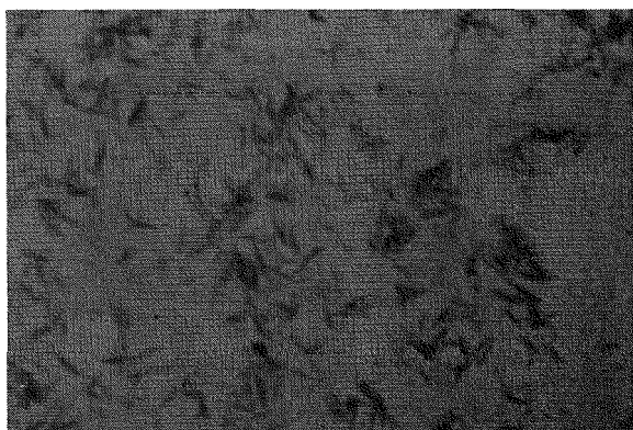
Fig. 33—Alumina Sol, 50,000X
