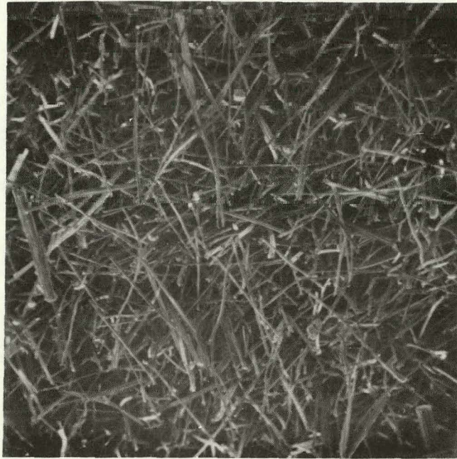
FIGURE 23. FIBER AND 18666-88 GRAPHITE (5 w/o) POWDER VIEWED APPROXIMATELY PERPENDICULAR TO THE DEPOSIT SURFACE.
