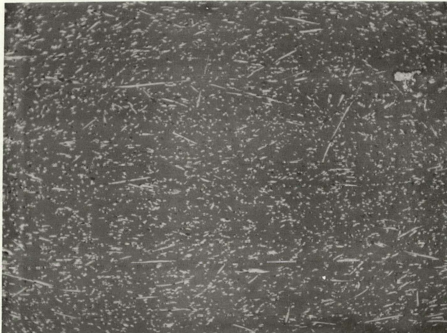
2E526 b. Section Perpendicular to the Plane of Deposition 100X
